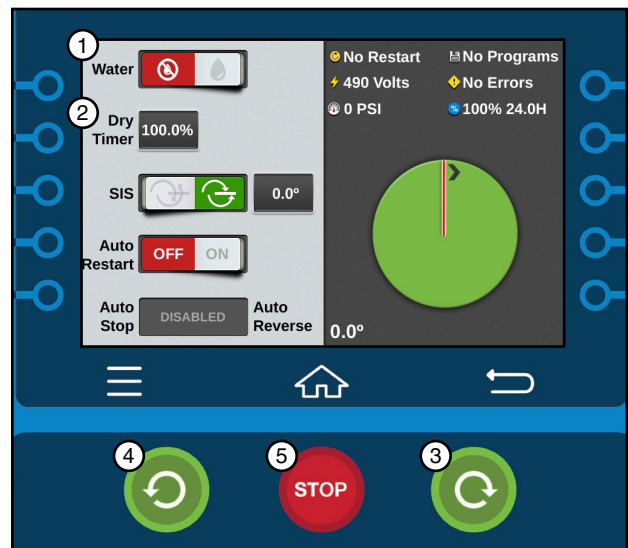
Figure 57-2 1. Water Off 2. Dry % Timer 3. Start Forward 4. Start Reverse 5. Stop
