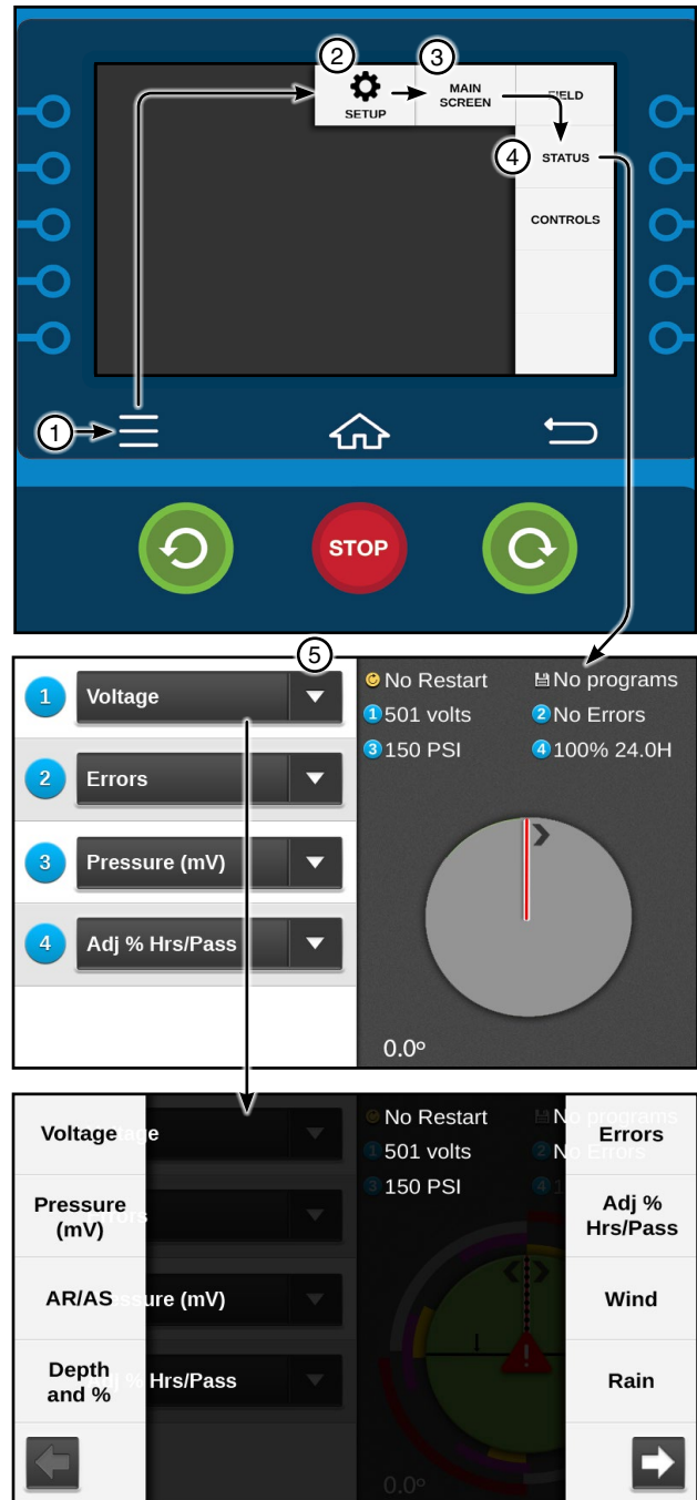
Figure 35-1 1. Menu 2. Setup 3. Main Screen 4. Status 5. Status Drop-Down Menu
