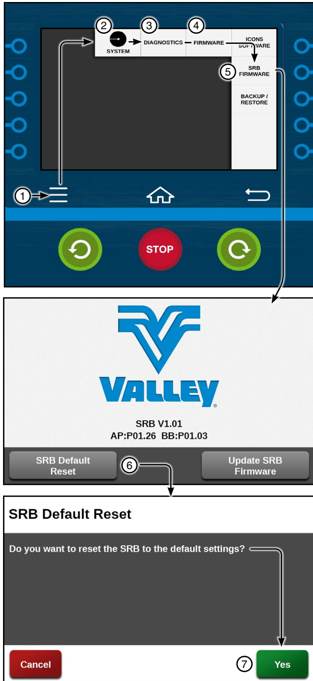
Figure 84-1 1. Menu 5. SRB Firmware 2. System 6. Update SRB Firmware 3. Diagnostics 7. Yes 4. Firmware
