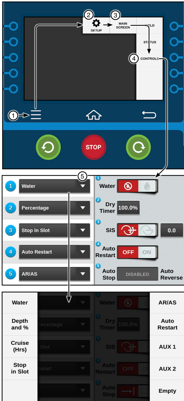
Figure 36-1 1. Menu 5. Control Drop-Down Menu 2. Setup 3. Main Screen 4. Controls
