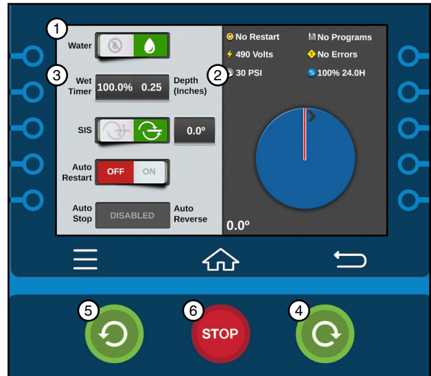
Figure 57-1 1. Water On 2. Depth 3. Wet % Timer 4. Start Forward 5. Start Reverse 6. Stop
