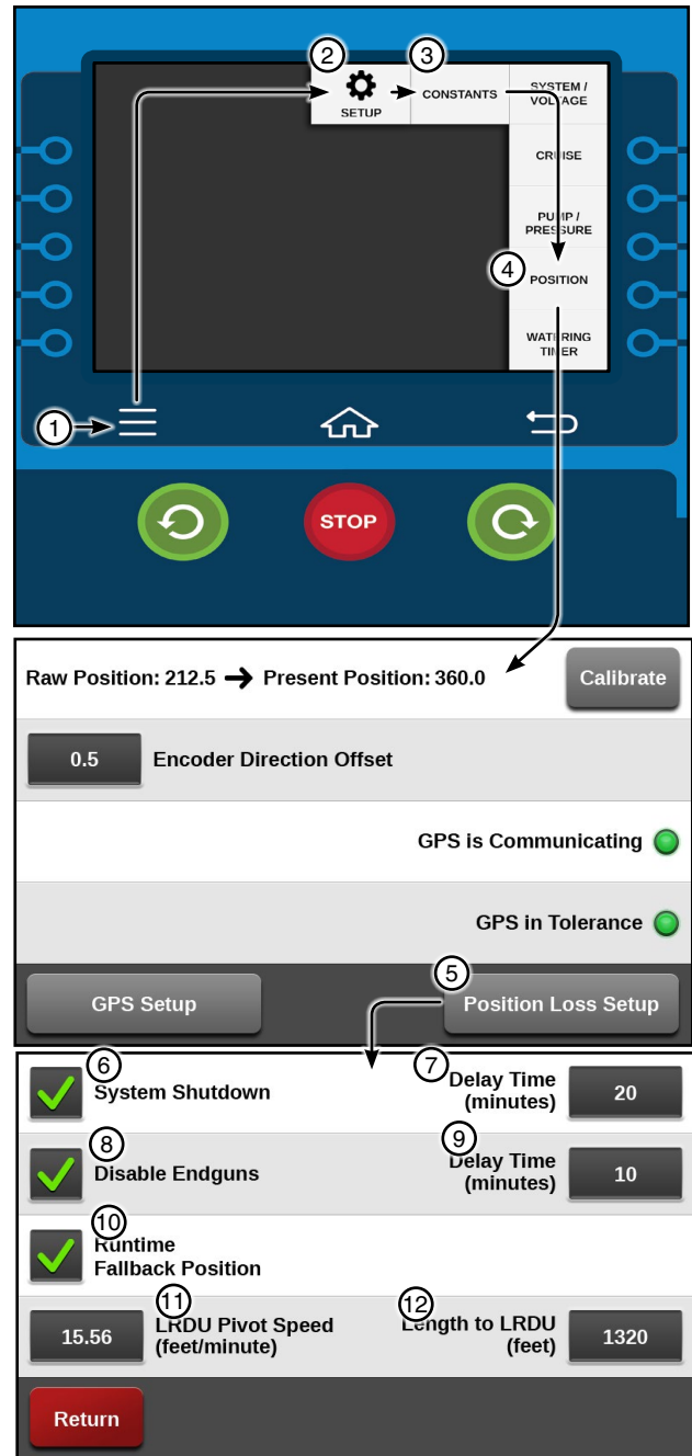
Figure 47-1 1. Menu 7. System Shutdown Delay 2. Setup 8. Disable End Guns 3. Constants 9. Disable End Guns Delay 4. Position 10. Fallback Position 5. Position Loss 11. LRDU Pivot Speed 6. System Shutdown 12. Length to LRDU
