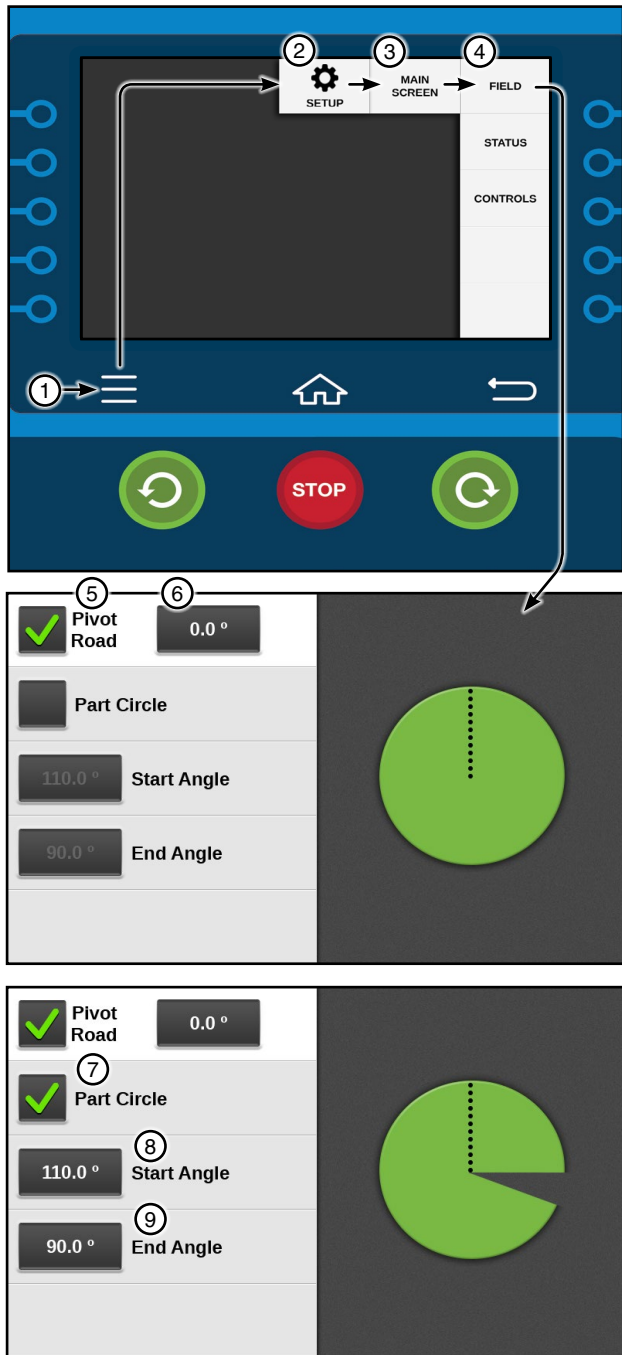
Figure 34-1 1. Menu 2. Setup 3. Main Screen 4. Field 5. Pivot Road Checkbox 6. Pivot Road Position 7. Part Circle Checkbox 8. Start Angle 9. End Angle
