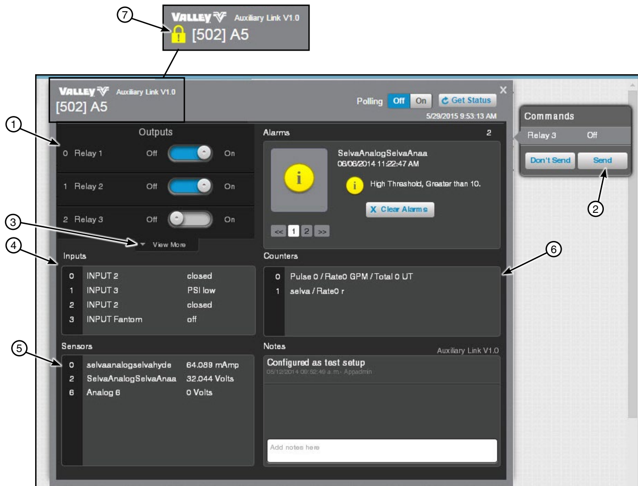
Figure 267-1 1. Outputs 5. Sensors 2. Commands List Dialog Send Button 6. Counters 3. View More/View Less 7. Remote Lock 4. Inputs
