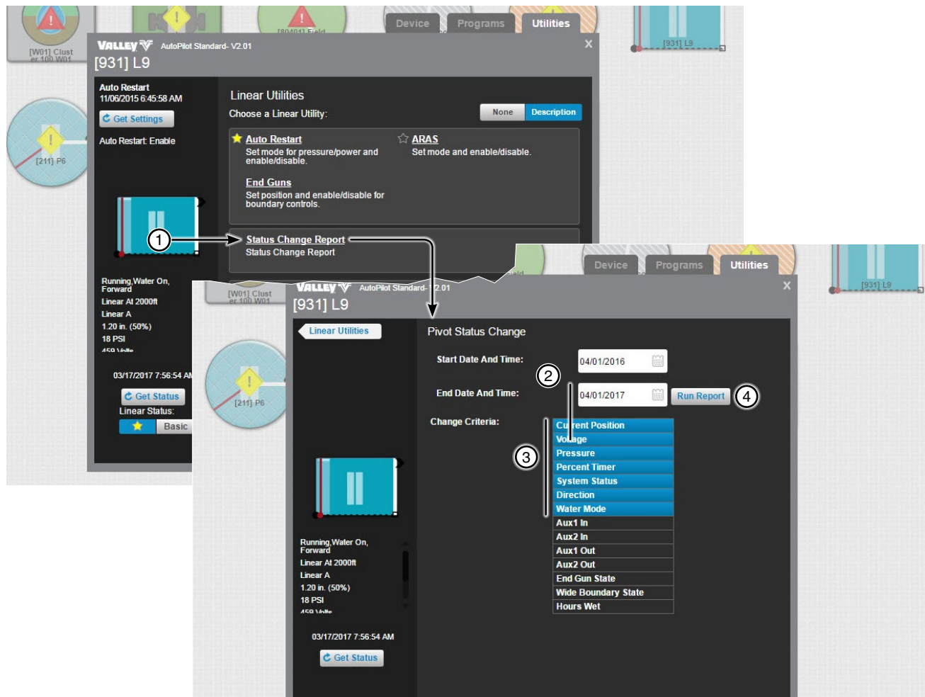
Figure 221-1 1. Click Status Change Report 2. Select Date Range 3. Select Change Criteria 4. Click Run Report
