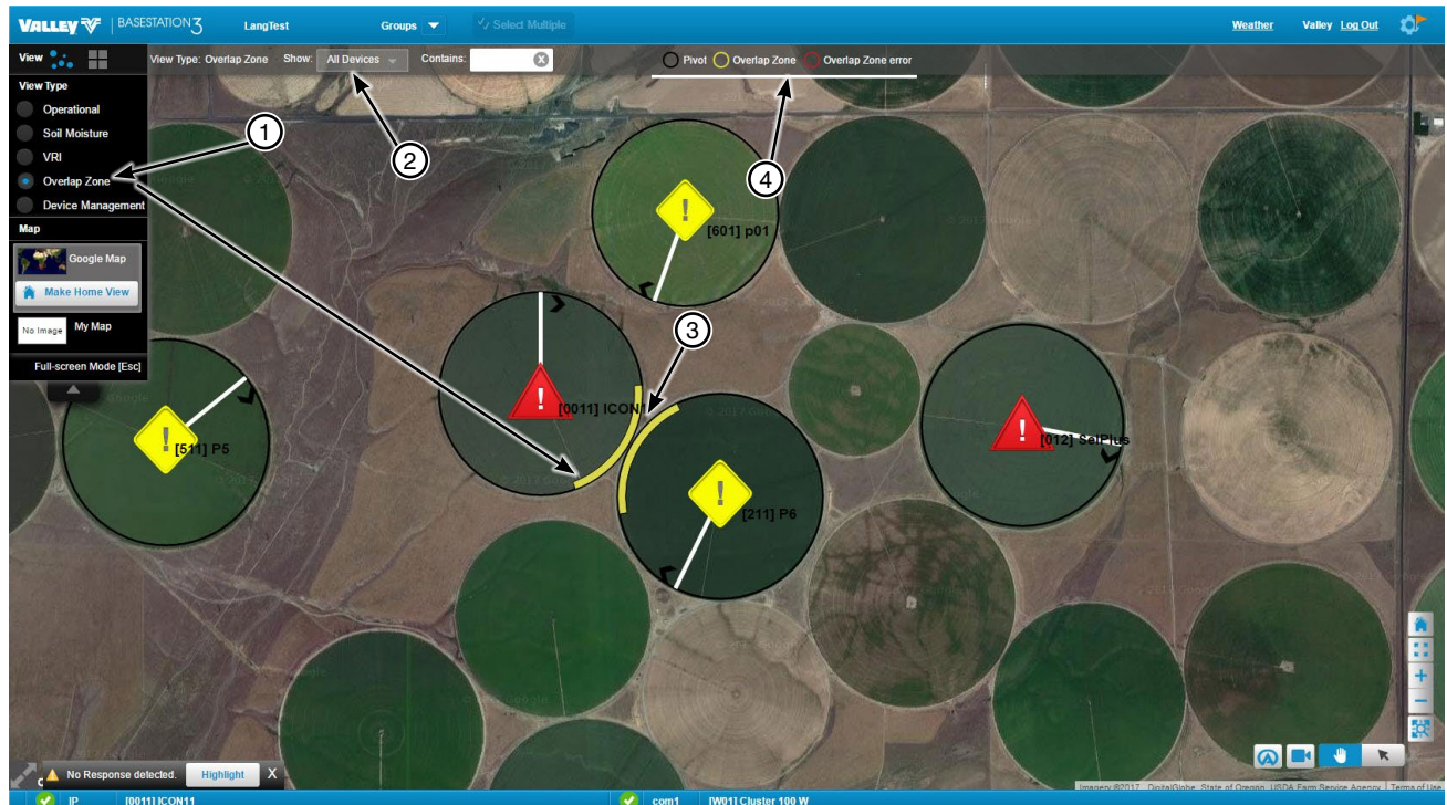
Figure 29-1 1. Overlap Zone Selected 2. Show Devices 3. Device Showing Status 4. Overlap Zone Status Key
