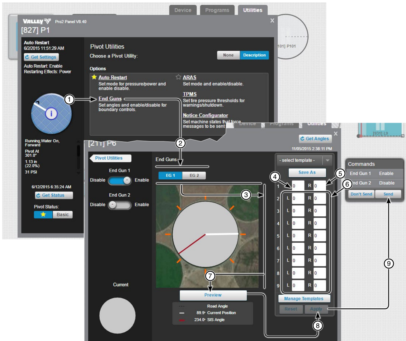
Figure 247-1 1. Click End Gun 2. Select the End Gun to Change 3. Determine Which Sequence Number to Change 4. Enter the Left Angle 5. Enter the Right Angle 6. Enter Angles in Other Sequences as Required 7. Click Preview 8. Click Apply 9. Click Send
