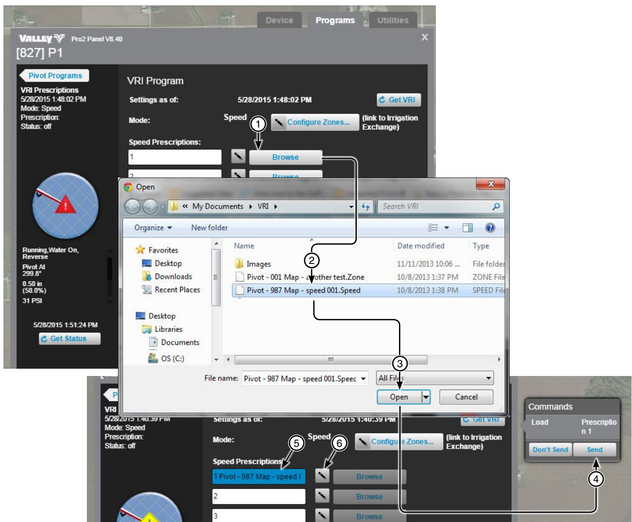
Figure 231-1 1. Click Browse 2. Select the Prescription File 3. Click Open 4. Click Send 5. File Name Reference 6. Change Button
