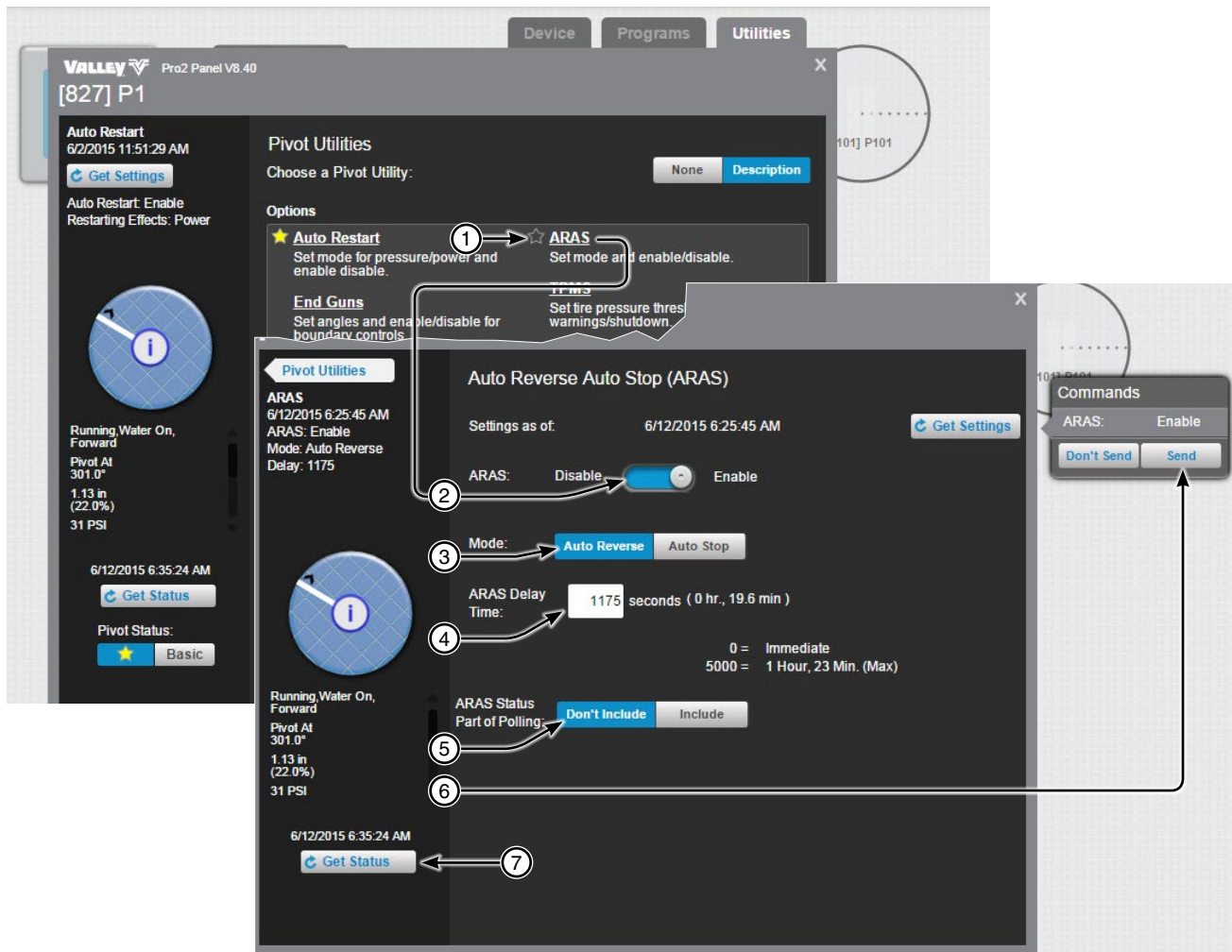
Figure 245-1 1. Click ARAS 2. Drag or Click Switch to Enable 3. Select the Mode 4. Enter the Engagement Delay Time 5. Select the ARAS Polling Status 6. Click Send 7. Click Get Status
