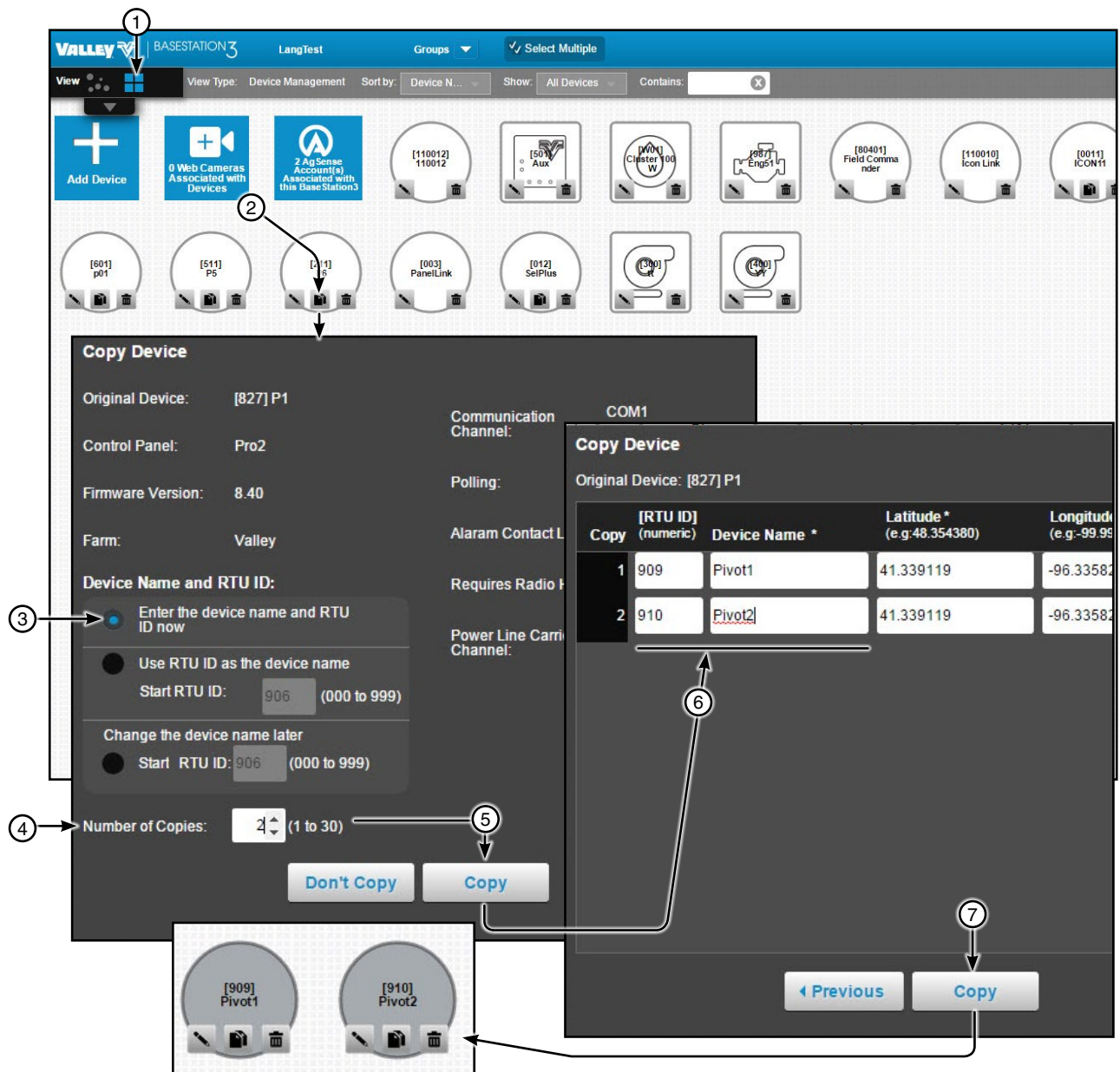
Figure 116-1 1. Tile View Device Management Screen 2. Click Copy 3. Enter the Device Name and RTU ID Now 4. Set Number of Copies 5. Click Copy 6. Enter RTU ID and Device Name 7. Click Copy
