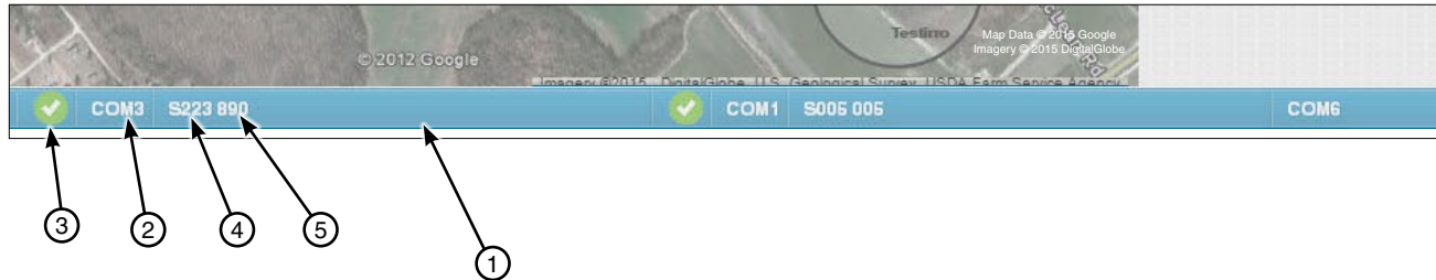
Figure 34-1 1. Communications Bar 2. Communications Channel 3. Status Transaction Activity Icon 4. Device Name 5. Device RTU ID
