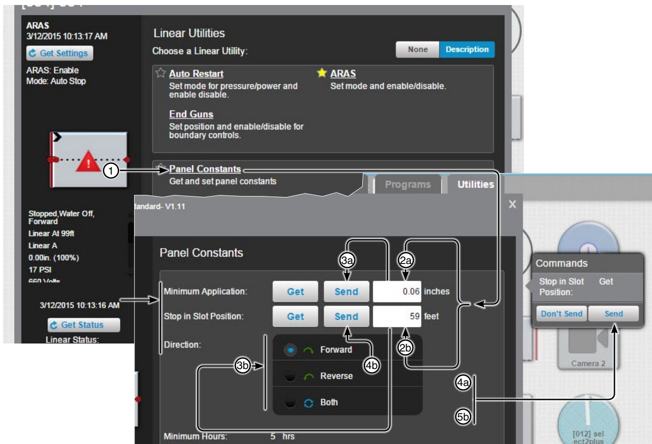
Figure 223-1 Minimum Application 1. Click Panel Constants 2a. Enter a value 3a. Click Send 4a. Click Send
