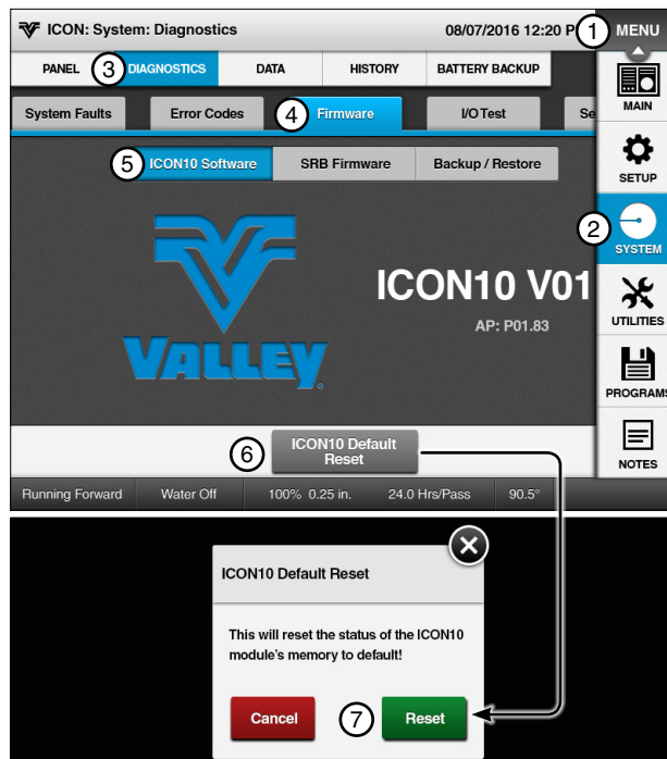
Figure 81-1 1. Menu 2. System 3. Diagnostics 4. Firmware 5. ICON10 Software 6. ICON10 Default Reset 7. Reset
