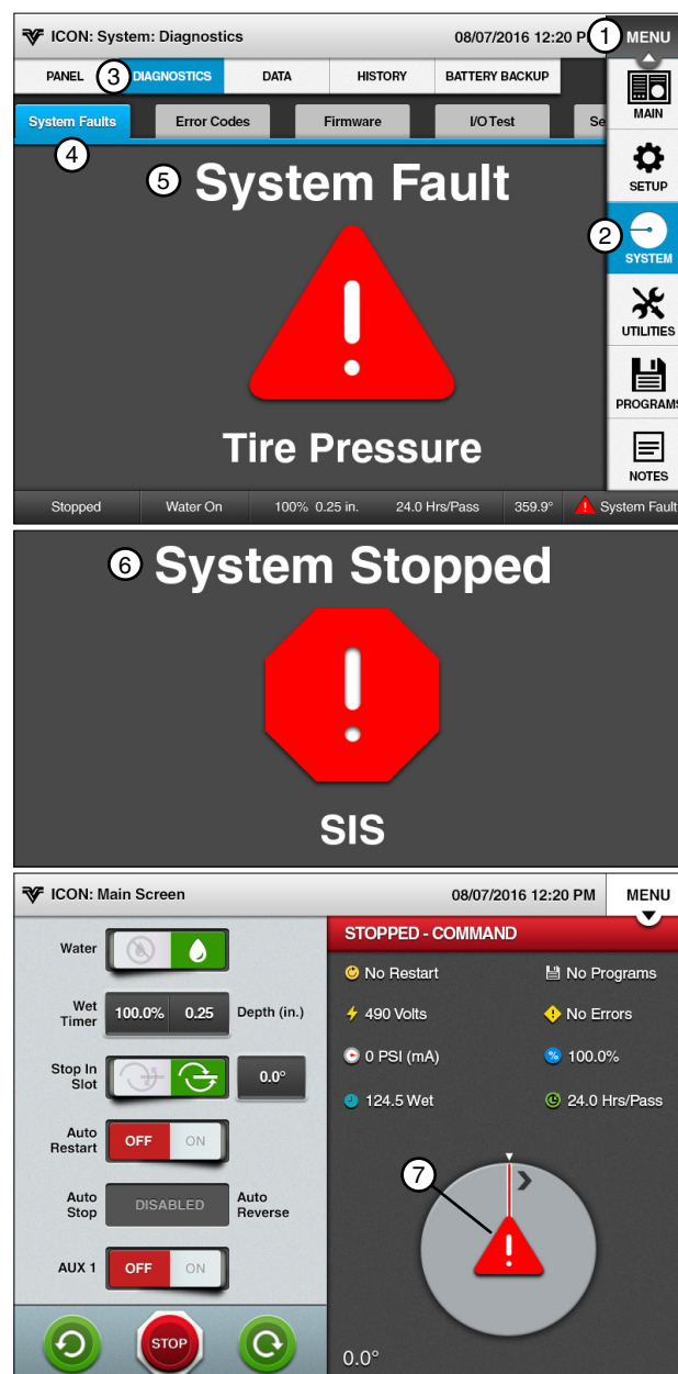
Figure 57-1 1. Menu 5. System Fault 2. System 6. System Stopped 3. Diagnostics 7. Fault Icon 4. System Faults
