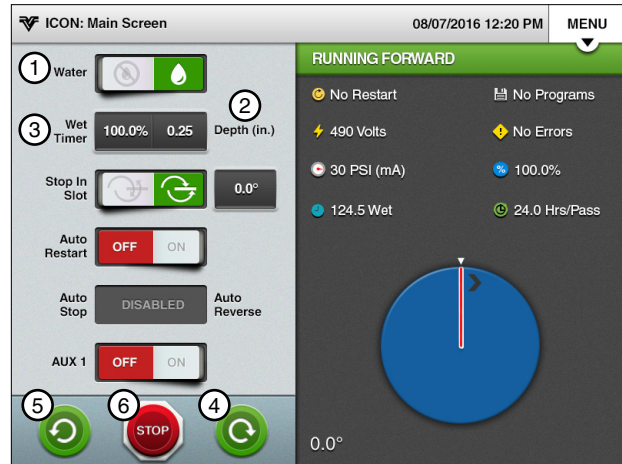
Figure 54-1 1. Water On 2. Depth 3. Wet % Timer 4. Start Forward 5. Start Reverse 6. Stop
