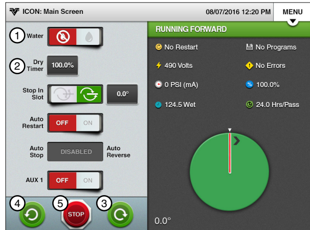
Figure 54-2 1. Water Off 2. Dry % Timer 3. Start Forward 4. Start Reverse 5. Stop
