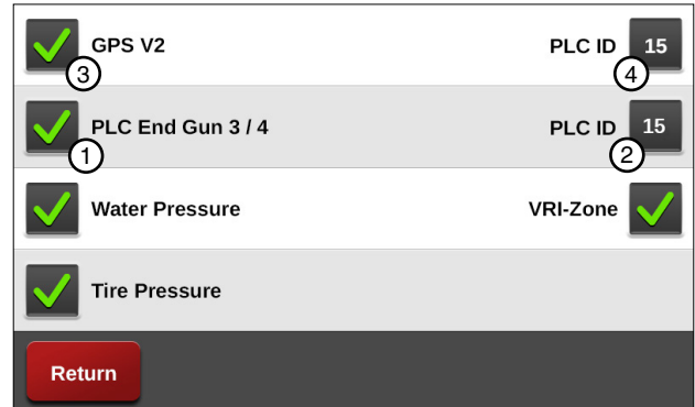
Figure 51-1 PLC Setup Screen 1. PLC End Gun 3 / 4 Checkbox 2. PLC End Gun 3 / 4 PLC ID 3. GPS V2 Checkbox 4. GPS V2 PLC ID
