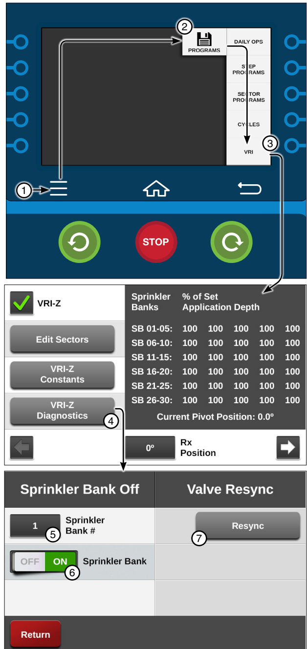
Figure 169-1 1. Menu 2. Programs 3. VRI 4. VRI-Z Diagnostics 5. Sprinkler Bank # 6. Sprinkler Bank Switch 7. Resync
