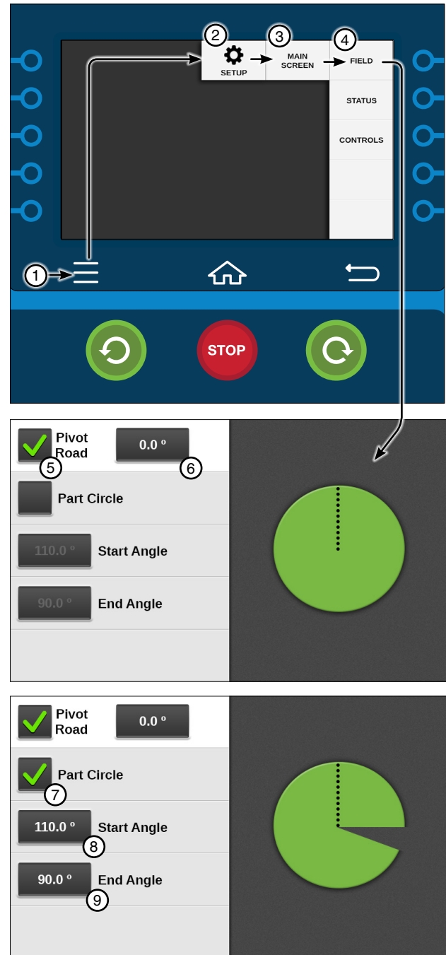
Figure 21-1 1. Menu 6. Pivot Road Position 2. Setup 7. Part Circle Checkbox 3. Main Screen 8. Start Angle 4. Field 9. End Angle 5. Pivot Road Checkbox
