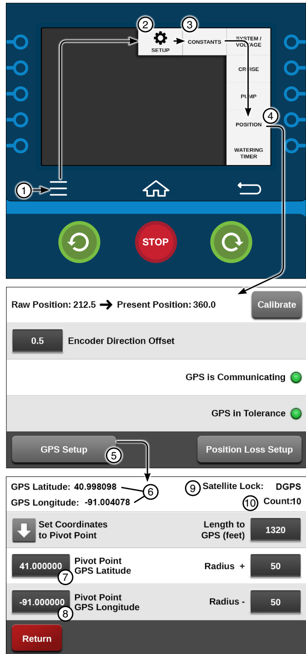
Figure 38-1 1. Menu 2. Setup 3. Constants 4. Position 5. GPS Setup 6. Current Position 7. Pivot Point GPS Latitude 8. Pivot Point GPS Longitude 9. Satellite Lock 10.Count
