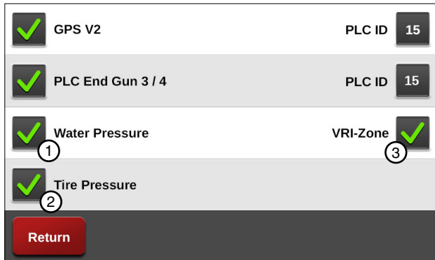
Figure 52-1 PLC Screen 1. Water Pressure Checkbox 2. Tire Pressure Checkbox 3. VRI-Zone Checkbox
