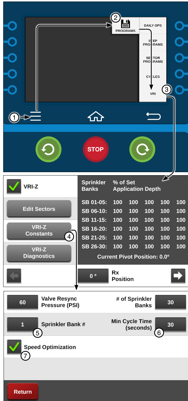
Figure 168-1 1. Menu 5. Sprinkler Bank # 2. Programs 6. Min Cycle Time 3. VRI 7. Speed Optimization 4. VRI-Z Constants
