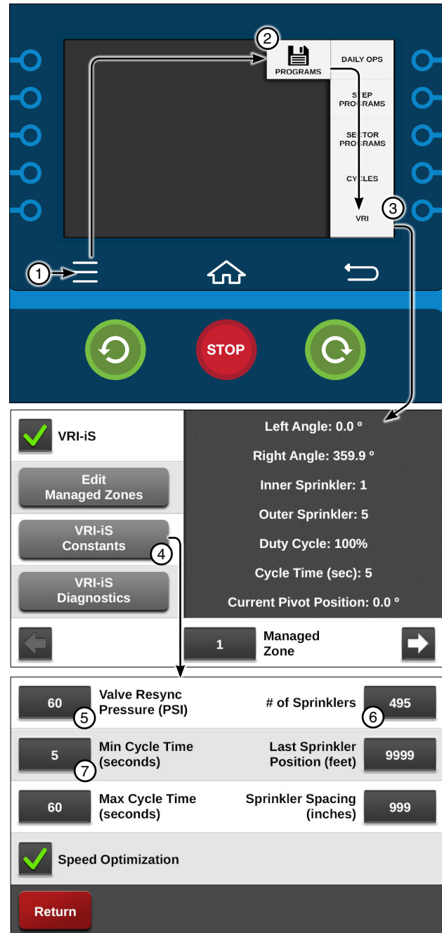
Figure 176-1 1. Menu 5. Valve Resync Pressure 2. Programs 6. # of Sprinklers 3. VRI 7. Min Cycle Time 4. VRI-iS Constants
