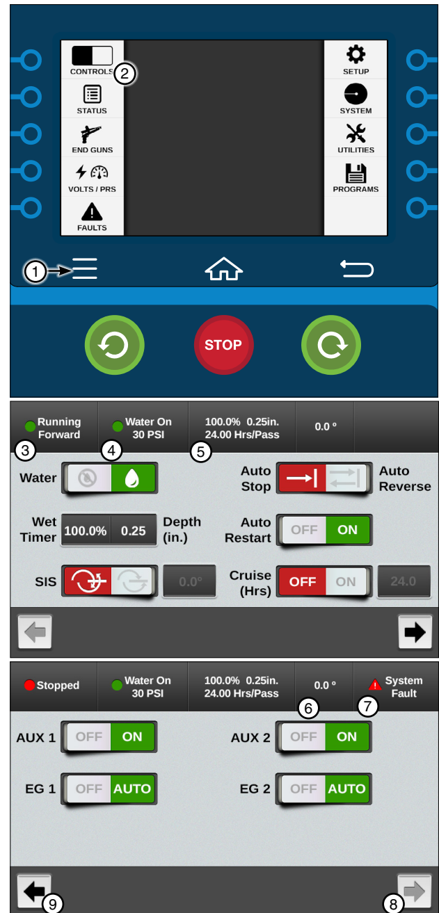
Figure 11-1 1. Menu 6. Position 2. Controls 7. System Fault 3. Machine Status / Direction 8. Next 4. Water On / Pressure 9. Previous 5. % Timer / Hrs/Pass
