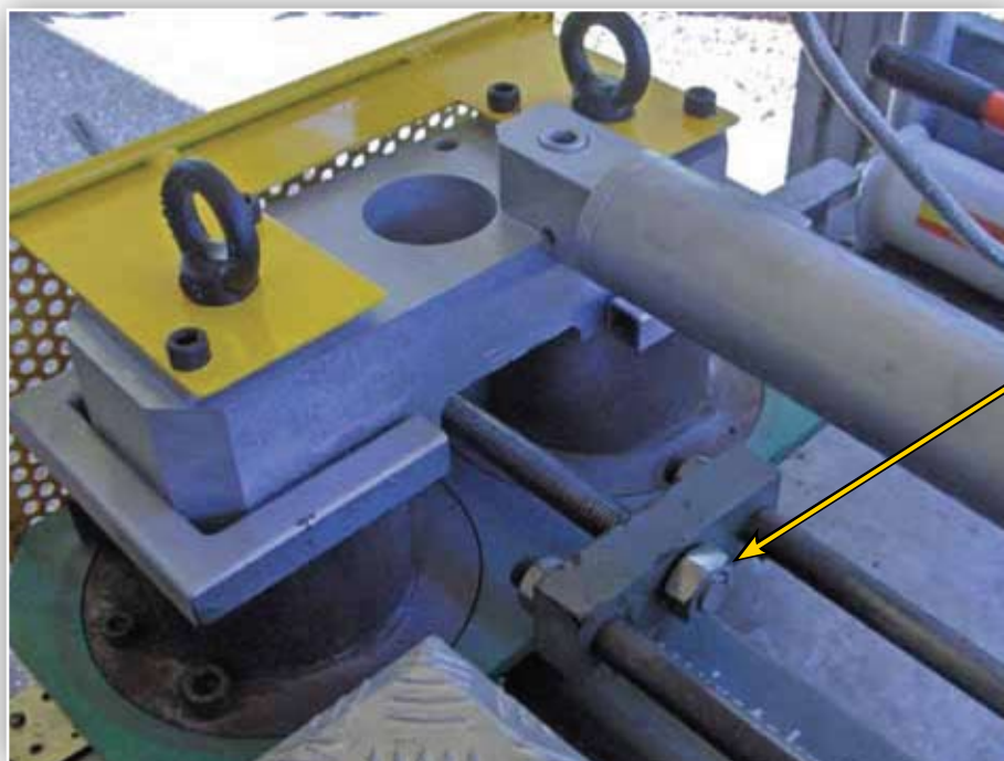
Figure 8: Attachment of End Fitting to Cross Bar
