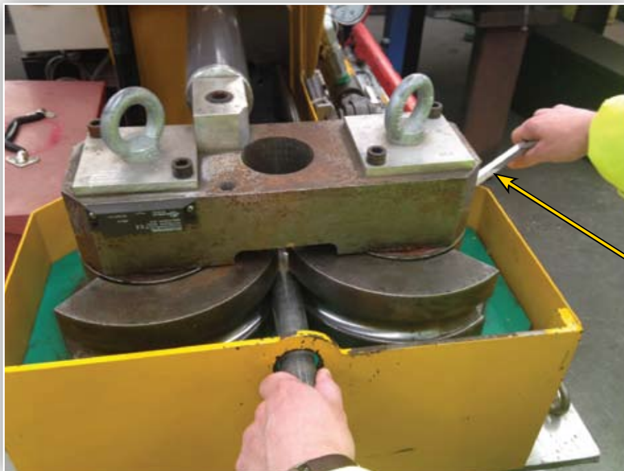
Figure 9: Initial positioning of the end fitting
