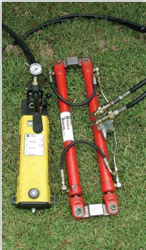
Figure 4: Hand Pump & Tension Unit
