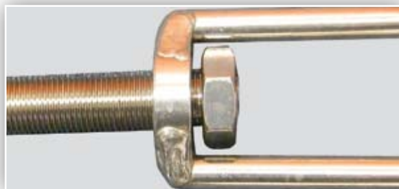
Figure 7: End Fitting with Nut Attached
