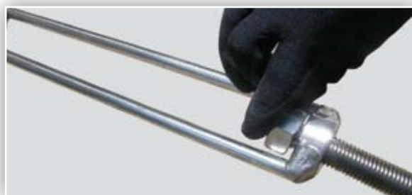
Figure 6: Attachment of End Fitting Nut
