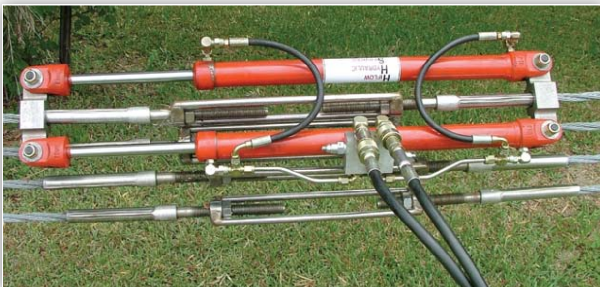
Figure 8: Tension Unit Connection to Tension Bay
