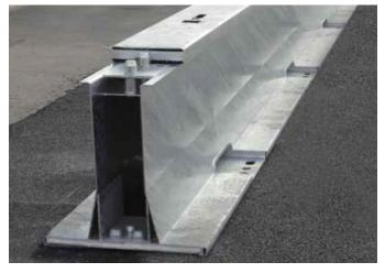
HighwayGuard™ LDS is a MASH 16 TL-3 & TL-4 compliant steel safety barrier. The 6m single barrier section, with the unique T-Connector provides quicker installation, removal and separation of barrier sections. It also offers the ability to remove sections within a run to create access gaps, replace damaged sections or alter barrier runs.
