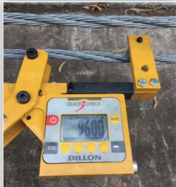
Checking Cable Tension with Dillon Meter
