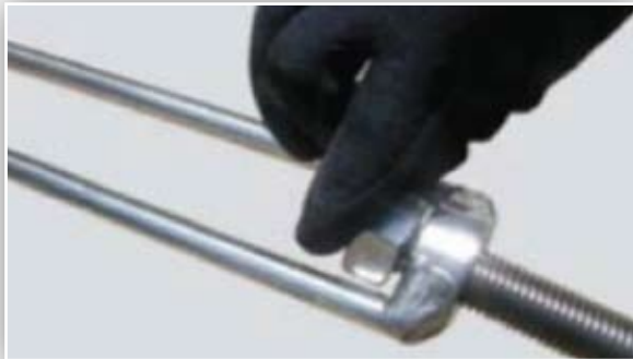
Attach nut to swaged fitting end
