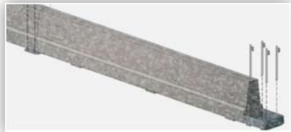
Full height terminals (male and female) anchoring positions are indicated below.
