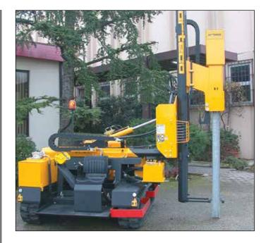
The self-propelled Ingal Heavy Duty Post Driver 800HD is specially designed for large-scale guardrail projects that require a heavier and more powerful machine. A few simple commands move the machine from the 'shipping' position to the 'working' position reducing valuable set-up time.
