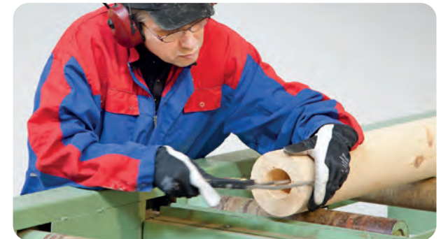
The lower part of the shaft is milled exactly to fit the steel base.
