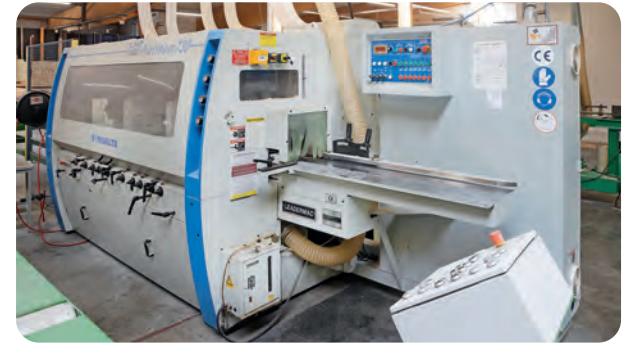
Using a CNC machine, round and conical poles are formed.
