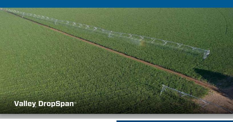
The Valley<sub>®</sub> DropSpan™ allows the outer spans of your center pivot to be dropped from the machine, so you can irrigate additional land adjacent to large obstructions at the edge of the field.
