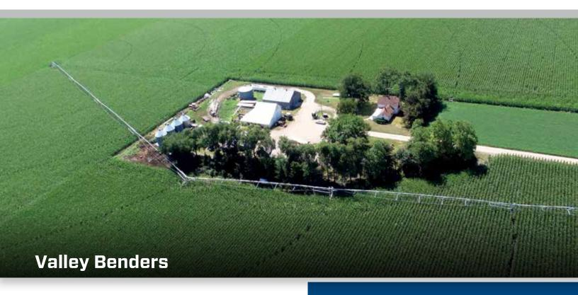
The Bender options maximize irrigated area at a low cost, allowing the outer portion of a pivot to continue moving even after fences, trees or other obstacles stop the inner portion.
