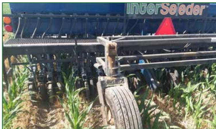
Lowell King of Fruita, CO is using his InterSeeder drill to place three rows of companions between each row of corn at approximately V4 stage.
