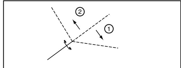
Figure 25-3 1. Forward Angle 2. Backward Angle
