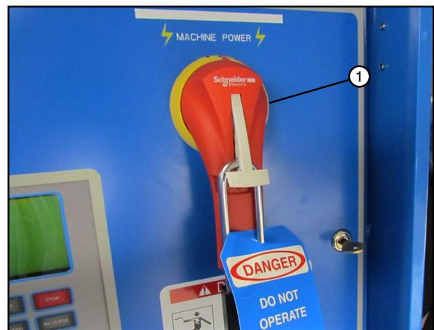
Figure 43-3 1. Main Power Disconnect Series
