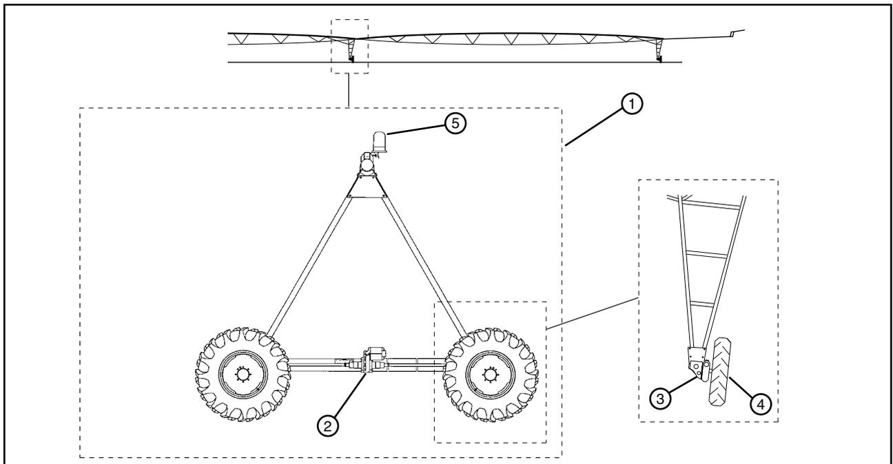
Figure 25-4 1. Drive Tower 2. Center Drive Gearbox 3. Wheel Gearbox 4. Tire And Wheel Assembly 5. Tower Box
