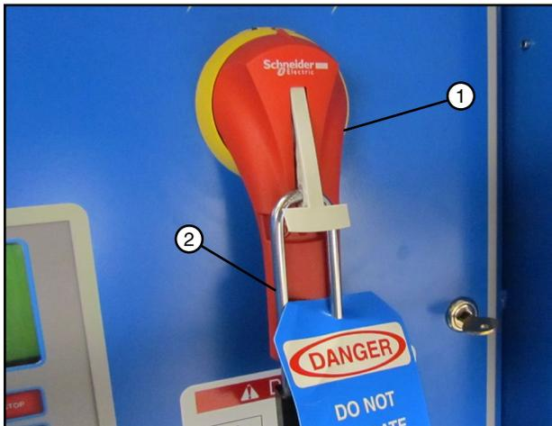
Figure 13-1 1. Main Power Disconnect
