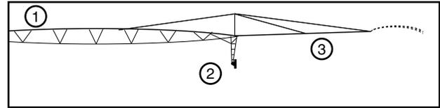
Figure 25-1 1. Span 2. Drive Unit 3. Overhang
