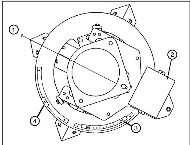
Figure 60-2 1. Pivot Direction 2. Control Box 3. End Gun Shut Off Ramp 4. Stop-In-Slot Ramp
