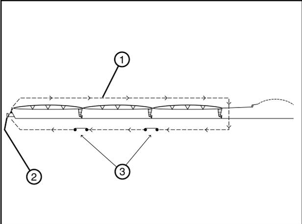
Figure 27-1 1. Safety circuit 2. Control panel 3. Safety Microswitch
