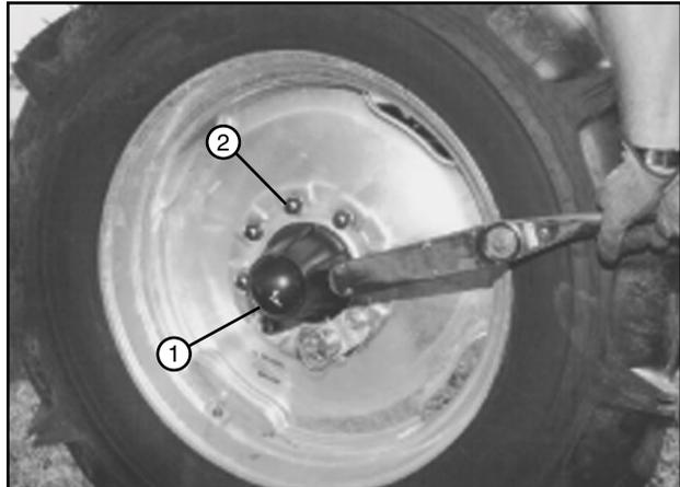
Figure 56-1 1. Grease Fitting
