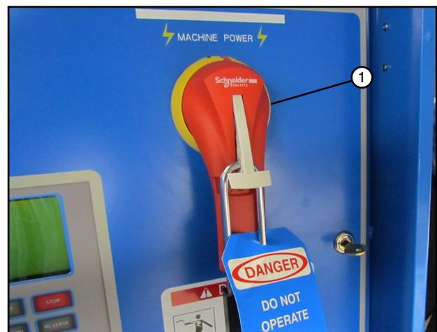
Figure 37-3 1. Main Power Disconnect
