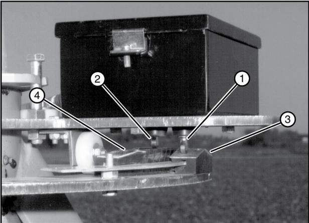
Figure 27-3 1. Stop In Slot Microswitch 2. End Gun Microswitch 3. Stop In Slot Ramp 4. End Gun Ramp
