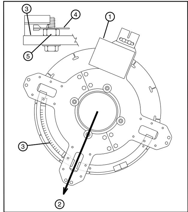
Figure 63-1 1. End Gun Control Box 4. Mounting Ring
