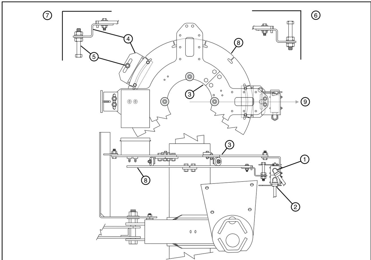
Figure 65-1 1. Auto Reverse Switch 4. Actuator Plate 7. Auto Forward Actuator Configuration
