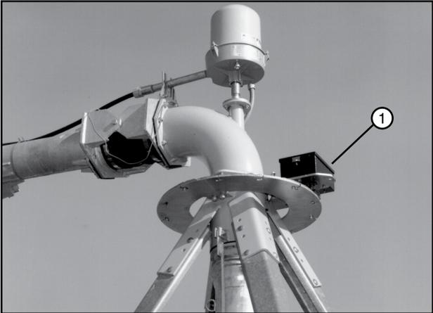
Figure 27-2 1. Stop In Slot / End Gun Control Box
