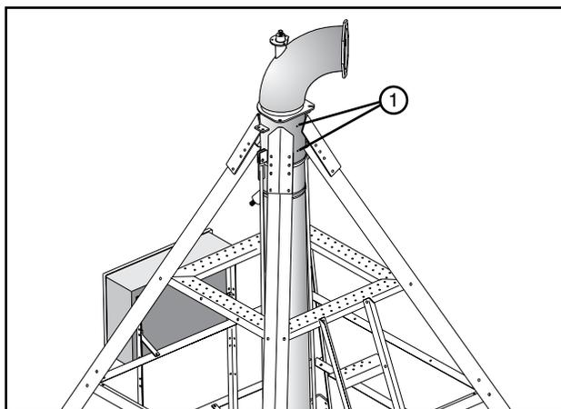
Figure 58-3 1. Grease Fitting
