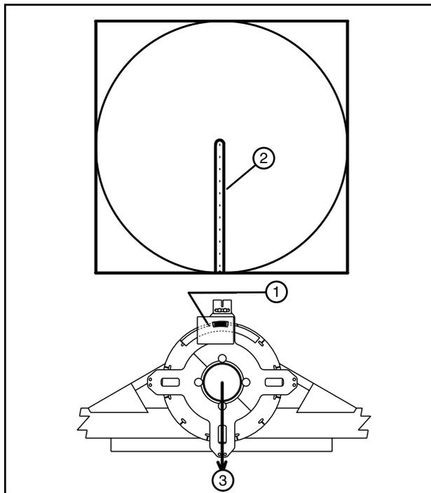
Figure 64-2 1. Stop-In-Slot Ramp 3. Pivot Road
