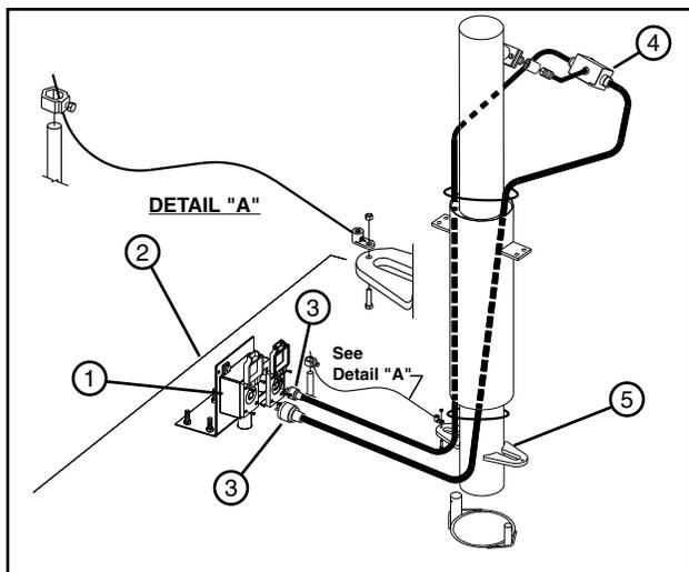
Figure 28-2 1. Electrical Receptacles 4. Electrical Box
