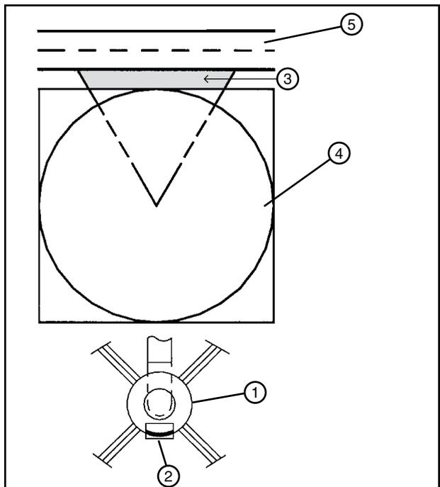
Figure 60-3 1. Pivot 2. Ramp Location 3. End Gun Shut Off Area 4. Field 5. Highway
