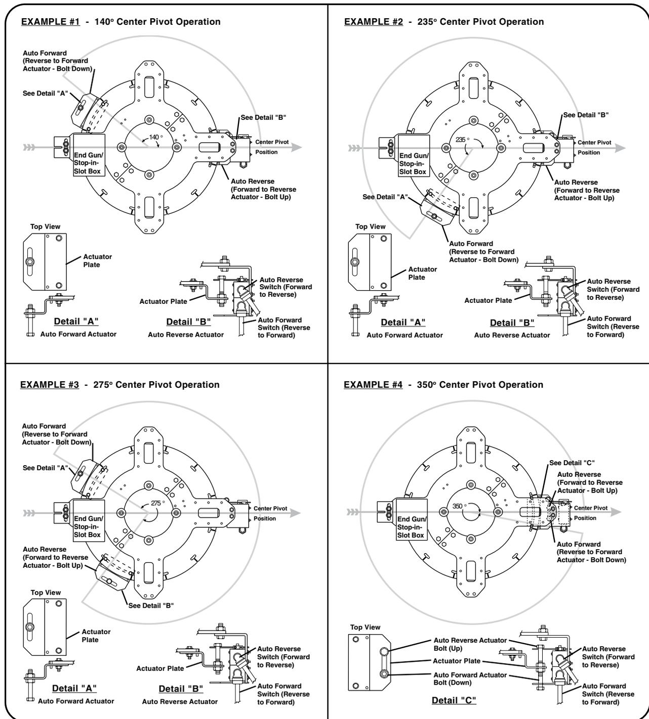
Figure 66-1 Detail "A" - Auto Forward ( Reverse to Forward Operation - Actuator Bolt Positioned Down)
