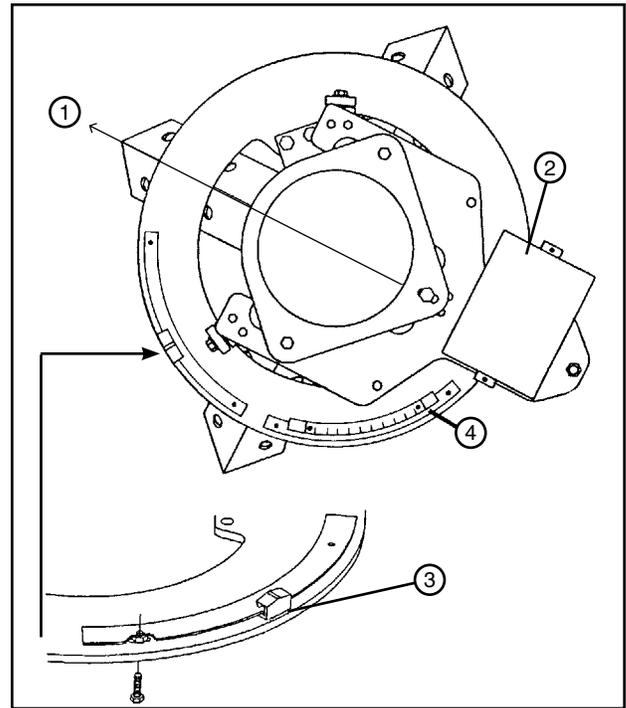
Figure 61-1 1. Pivot Direction 2. Control Box 3. Stop-In-Slot Ramp 4. End Gun Shut Off Ramp
