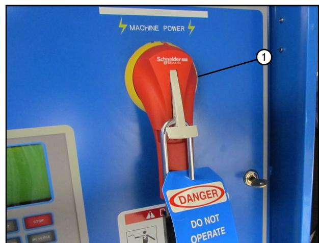
Figure 47-3 1. Main Power Disconnect Series 8000 Control Panel Shown
