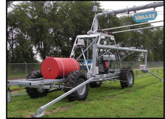
Figure 41-2 Swing Around Rainger Linear
