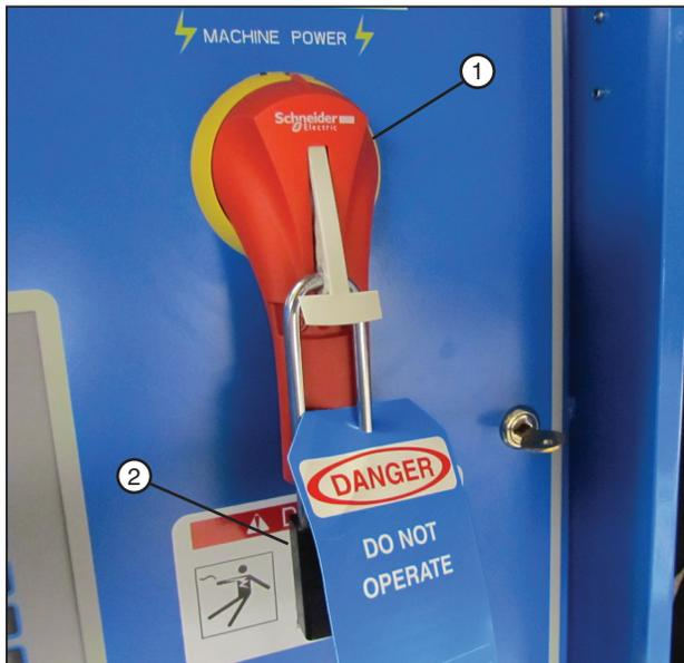
Figure 15-1 1. Main Power Disconnect
