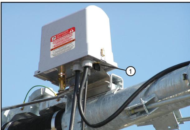
Figure 14-1 1. Disconnect Switch
