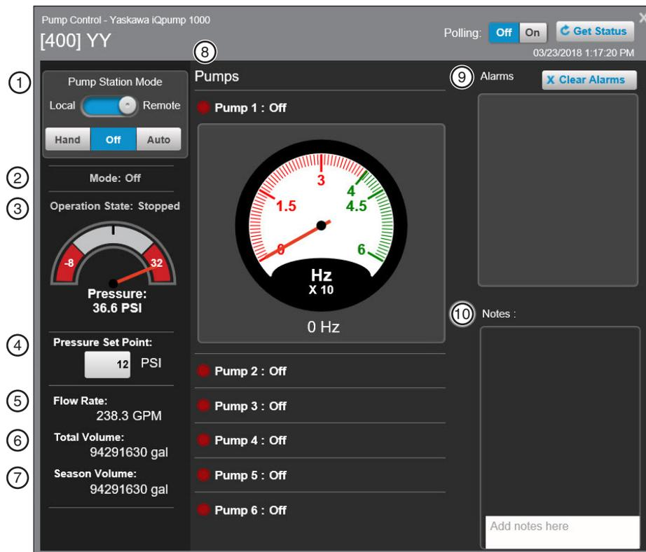
Figure 336-1 1. Pump Station Mode 6. Total Volume
