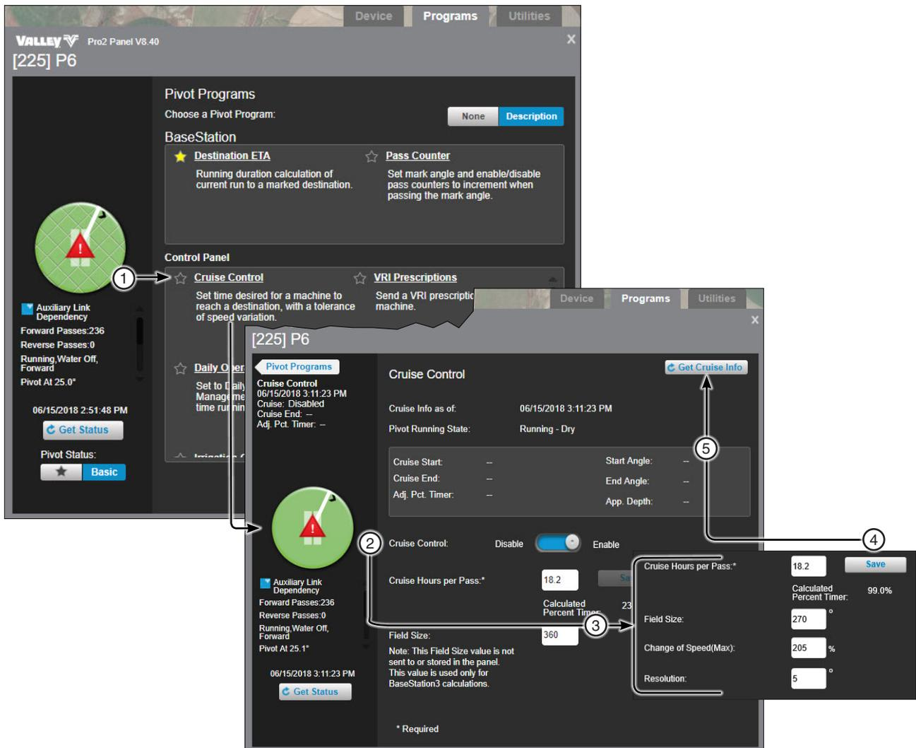
Figure 283-1 1. Cruise Control 2. Disable/Enable 3. Cruise Hours per Pass 4. Save 5. Get Cruise Info
