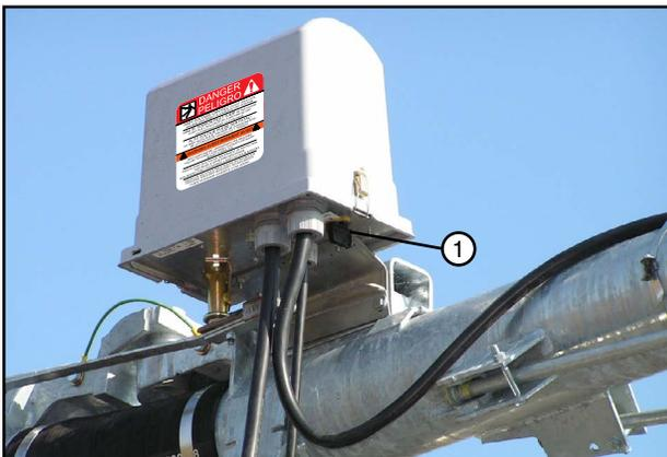
Figure 10-1 1. Disconnect Switch
