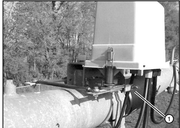
Figure 83-1 1. Tower box side of drive unit
