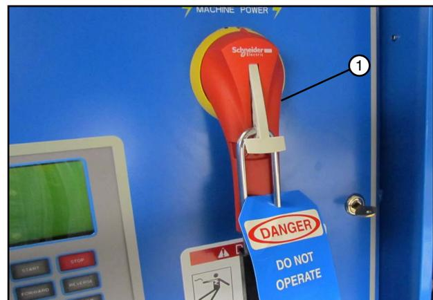
Figure 53-3 1. Main Power Disconnect
