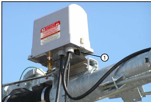
Figure 13-1 1. Disconnect Switch
