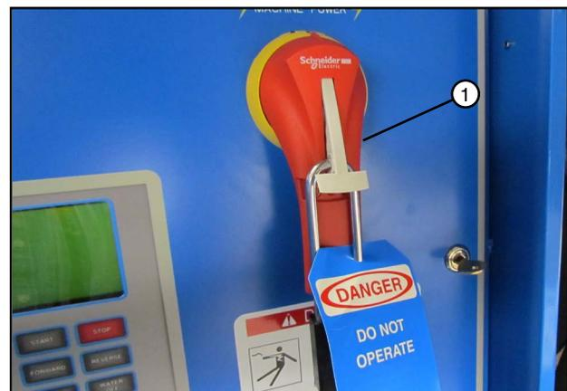
Figure 41-3 1. Main Power Disconnect
