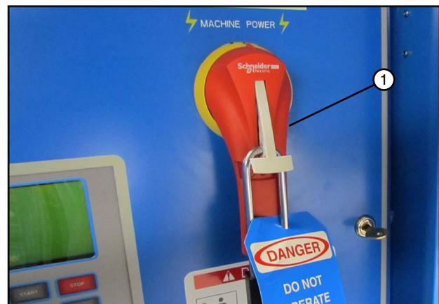
Figure 57-3 1. Main Power Disconnect
