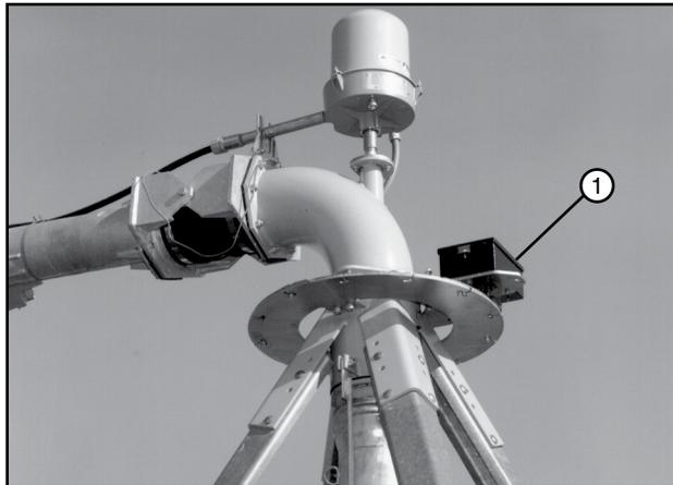
Figure 26-2 1. Stop In Slot / End Gun Control Box
