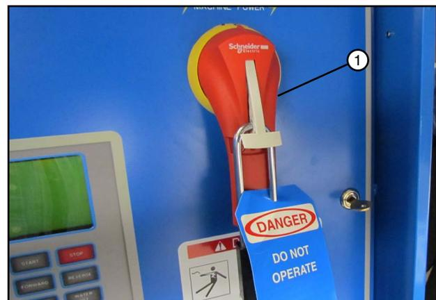
Figure 47-3 1. Main Power Disconnect
