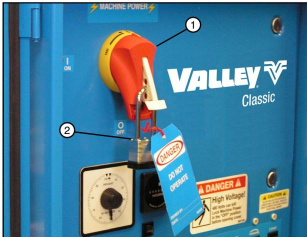
Figure 13-1 1. Main Power Disconnect
