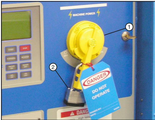
Figure 12-1 1. Main Power Disconnect
