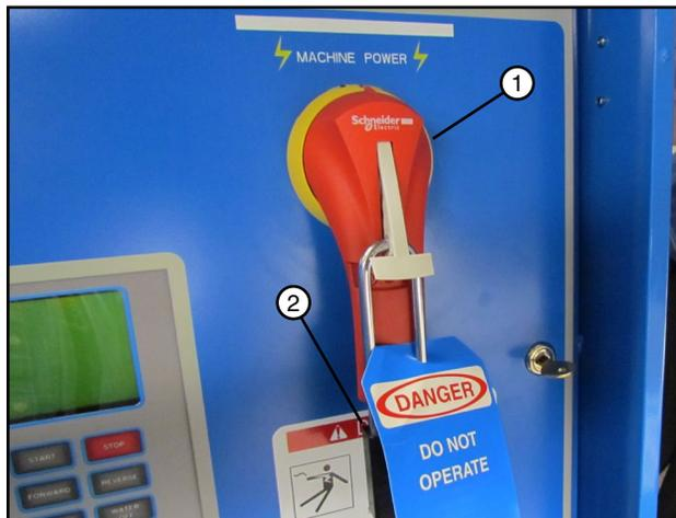
Figure 12-2 1. Main Power Disconnect
