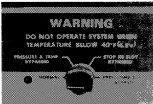
**BY-PASS SWITCH.** By-pass switch allows operator to by-pass the low pressure and temperature safety shutdown features and/or the Stop-In-Slot option if your VALLEY is equipped with these options. "NORMAL" position engages all shutdown features and will turn on the adjacent indicator light.
