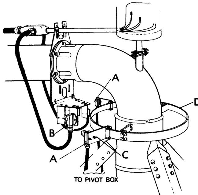
Auto-reverse switches (A), their mounting hardware and the two safety shut-down switches (B) are mounted as shown in the illustration. Each reversing switch has a back-up safety switch which will stop the system if the reversing switch or associated circuitry fails to achieve the direction change as planned.
