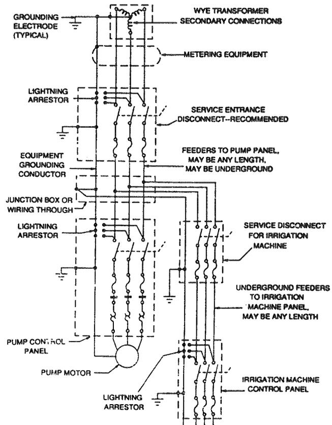
T Figure 1 - Recommended equipment and grounding for wye transformer secondary connections
