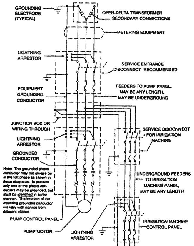
Figure 4 – Recommended equipment and grounding for a grounded phase, open-delta transformer secondary connections
