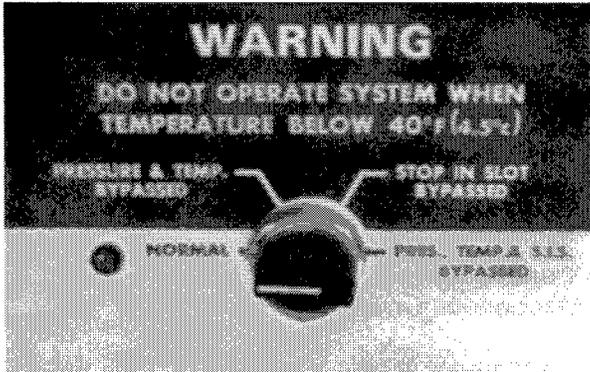
1. Turn **BY-PASS SWITCH** to position required. It may be necessary to select a by-pass function if:
