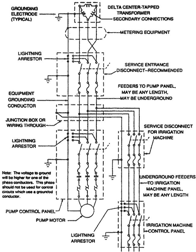
Figure 2 – Recommended equipment and grounding for delta center-tapped transformer secondary connections
