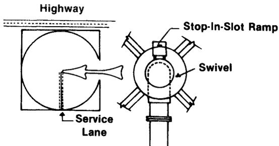
**NOTE:** Assure proper contact of ramp and switch roller. If necessary, insert spacer washer or 5/16" nut.
