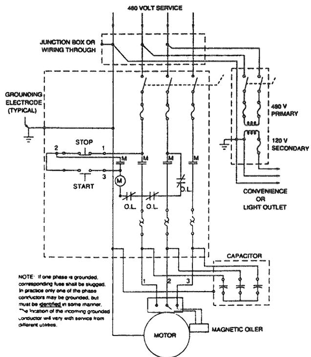
Figure 9 – Wiring diagram for capacitor installation and auxiliary equipment for 480 V service
