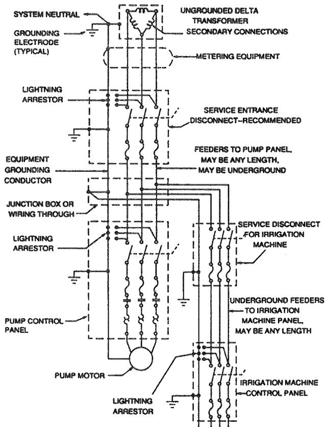
Figure 6 – Recommended equipment and grounding of three-phase, four-wire service when the transformer system is ungrounded
