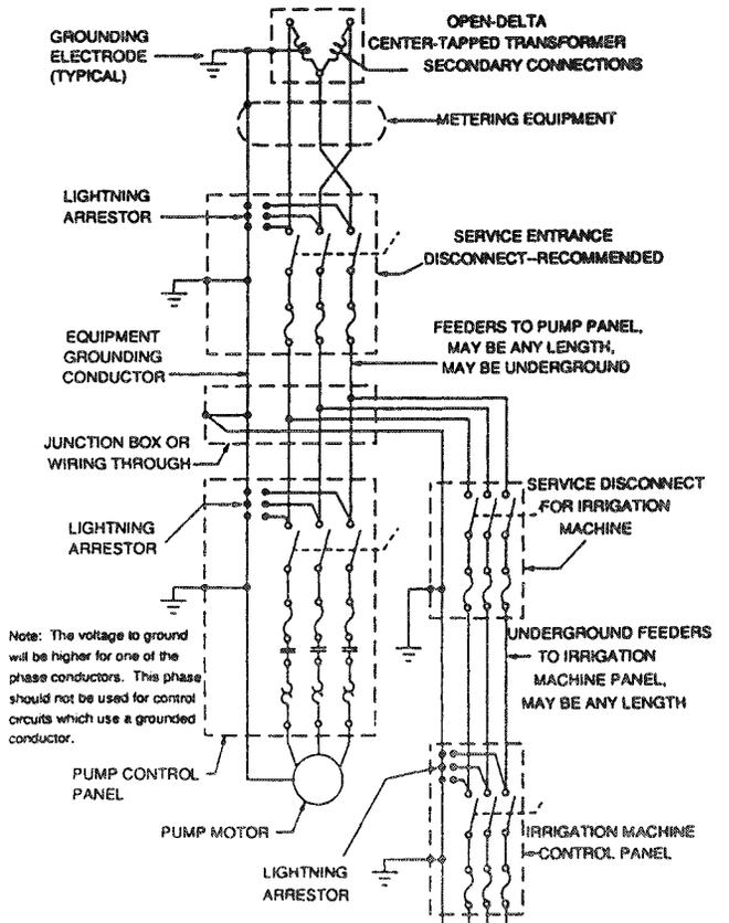
Figure 5 – Recommended equipment and grounding for open-delta, center-tapped transformer secondary connections
