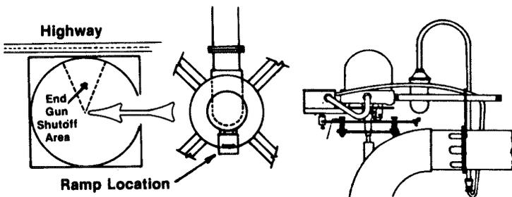
**NOTE:** Assure proper contact of ramp and switch roller. If necessary, insert spacer washer or 5/16" nut.
