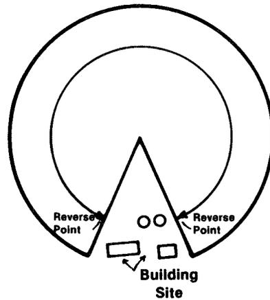
The Auto-Reverse Option can be adjusted to automatically change the system travel direction at predetermined locations, thereby causing the system to operate in a “windshield wiper” fashion.
