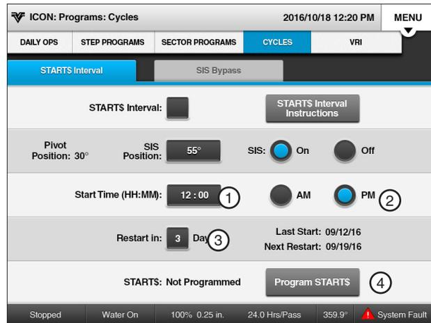
Figure 152-1 1. Start Time 2. AM or PM 3. Restart in (Days) 4. Program START\$
