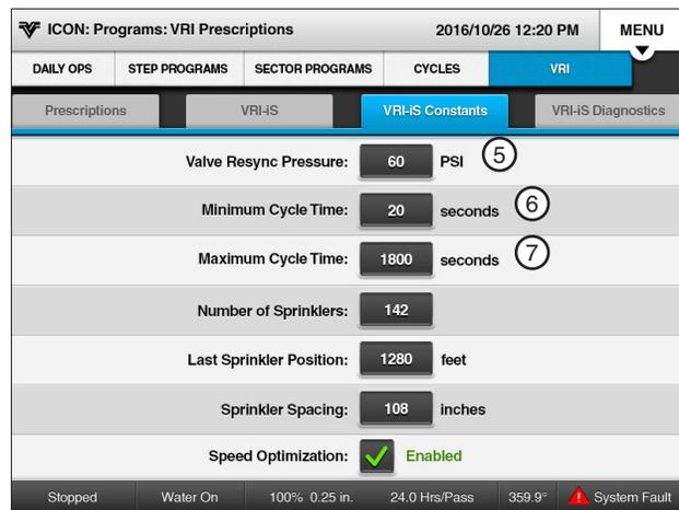
Figure 176-1 1. Menu 5. Valve Resync Pressure
