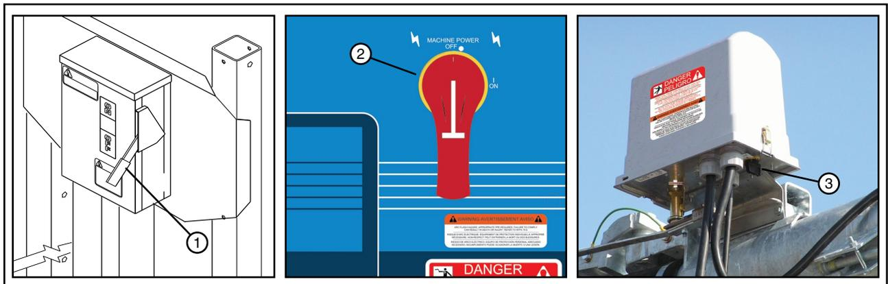
Figure 55-1 1. Main Service Disconnect Switch
