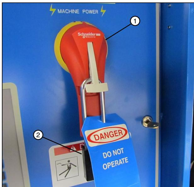
Figure 13-1 1. Main Power Disconnect
