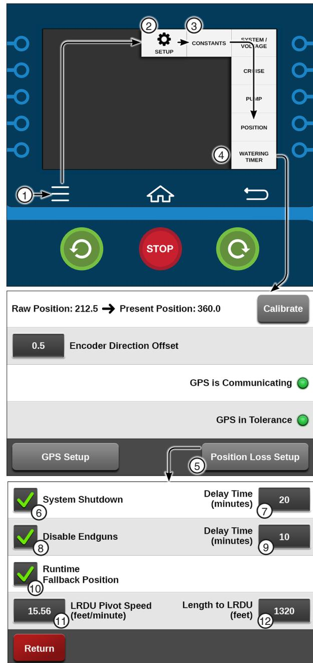
Figure 40-1 1. Menu 7. System Shutdown Delay
