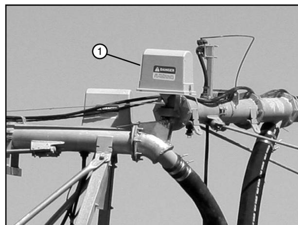
Figure 25-3 1. Corner Angle Sensor Box
