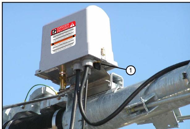
Figure 15-1 1. Disconnect Switch
