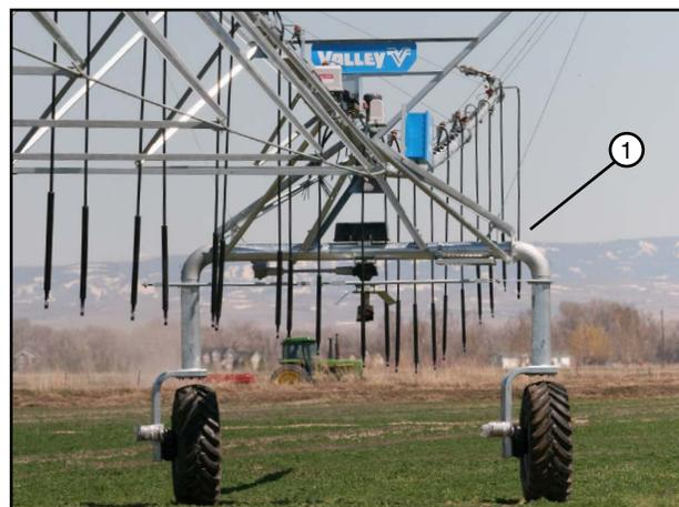
Figure 27-1 1. Steerable Drive Unit
