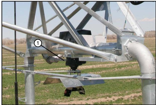
Figure 62-1 1. Steering Gearbox
