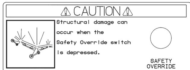
NEVER depress the override button longer than 3 to 5 seconds. The operator MUST inspect the entire machine between each start attempt. Repeated override start attempts can cause severe structural damage. Call the local Valley dealer should the machine fail to start.
