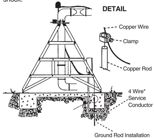
**\* IMPORTANT: All 480 volt AC power supply services MUST be a 4 conductor service. Three 480 Volt AC power lines and one ground conductor which is as large as the power carrying conductors for that service.**
