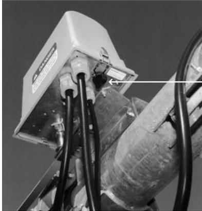
Stop the machine at any tower by turning the disconnect to the "OFF" position.
