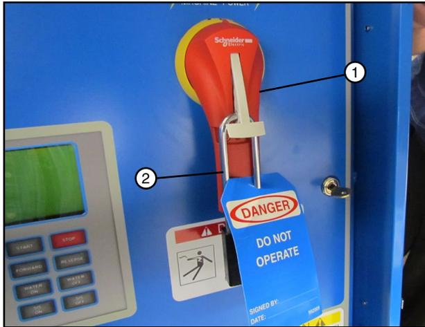
Figure 15-1 1. Main Power Disconnect
