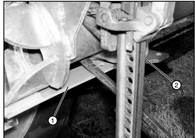
Figure 63-2 1. Steering Arm 2. Latch Plate
