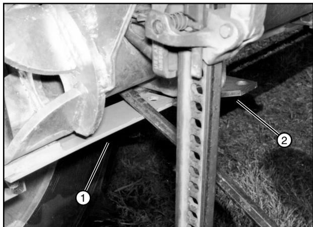
Figure 86-3 1. Steering Arm 2. Latch Plate
