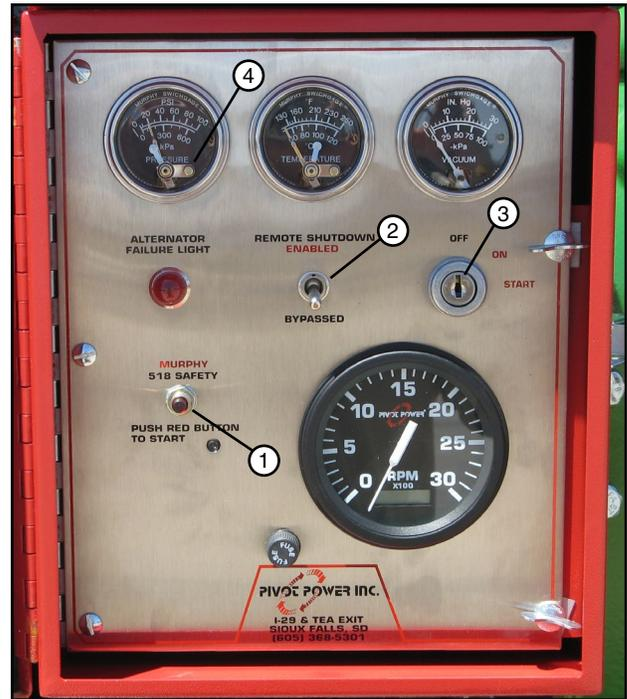
Figure 69-1 1. Safety Button 3. Engine Start Switch
