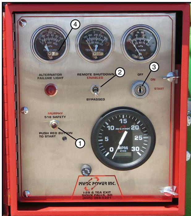
Figure 70-2 1. Safety Button 2. Toggle Switch 3. Engine Start Switch 4. Water Pressure Gauge Reset
