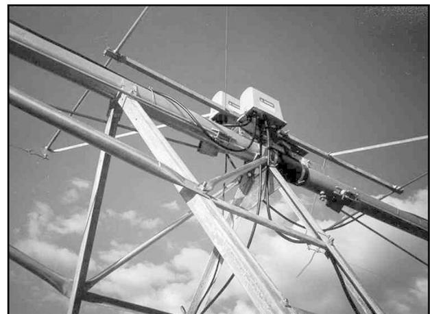
Figure 25-3 Floating alignment
