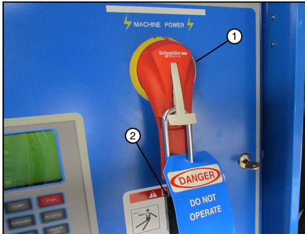
Figure 13-1 1. Main Power Disconnect
