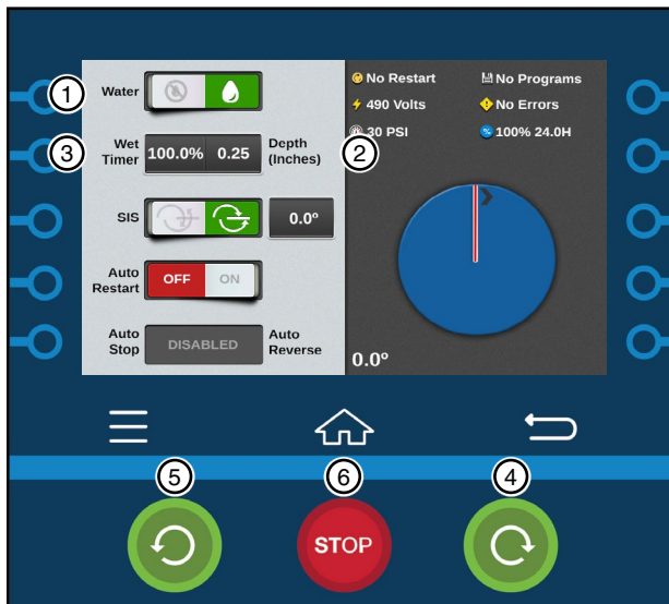
Figure 56-1 1. Water On 2. Depth 3. Wet % Timer 4. Start Forward 5. Start Reverse 6. Stop
