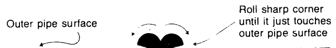
Cross section of butt fusion bead showing proper bead roll out (Bead size exaggerated for clarity)
