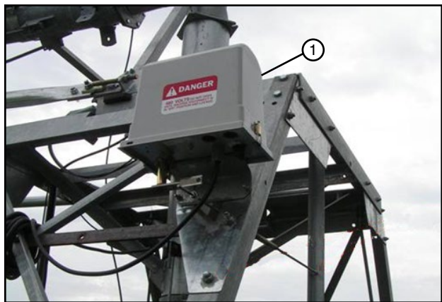
Figure 26-3 Swing Around Rainger Cart. 1. Cart Mounted Side Load Safety Box
