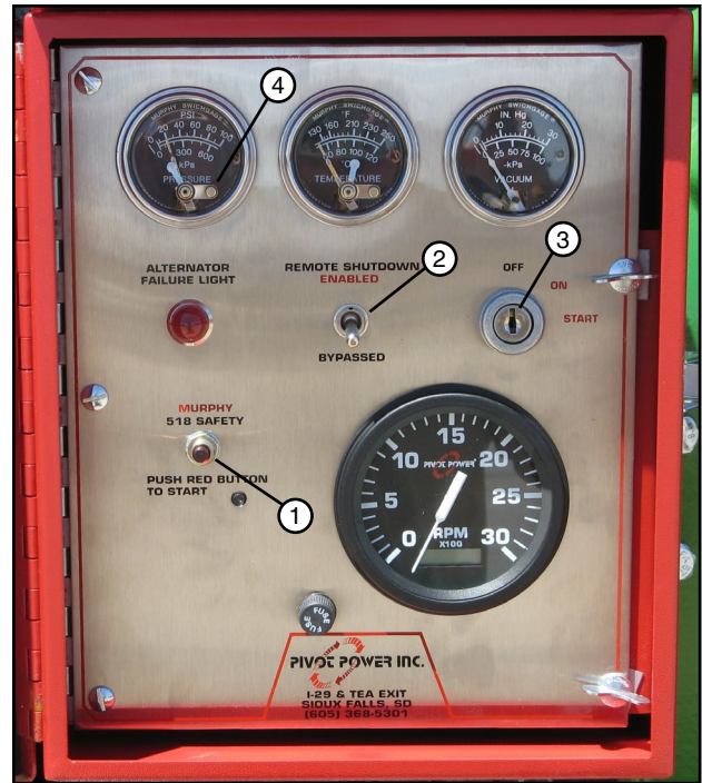
Figure 63-1 1. Safety Button 3. Engine Start Switch 2. Toggle Switch 4. Water Pressure Gauge Reset
