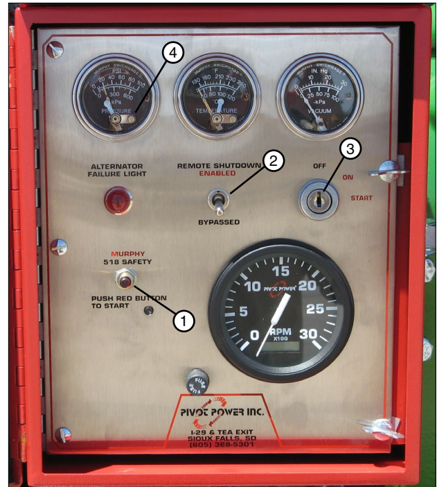
Figure 45-1 1. Safety Button 3. Engine Start Switch 2. Toggle Switch 4. Water Pressure Gauge Reset
