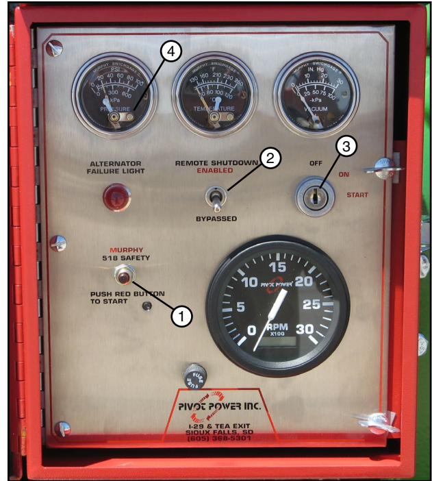
Figure 65-1 1. Safety Button 3. Engine Start Switch 2. Toggle Switch 4. Water Pressure Gauge Reset
