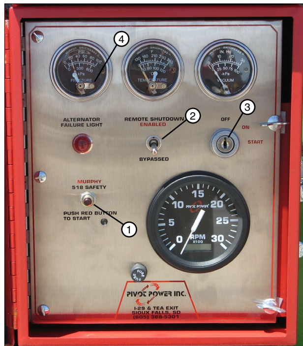
Figure 46-1 1. Safety Button 3. Engine Start Switch 2. Toggle Switch 4. Water Pressure Gauge Reset
