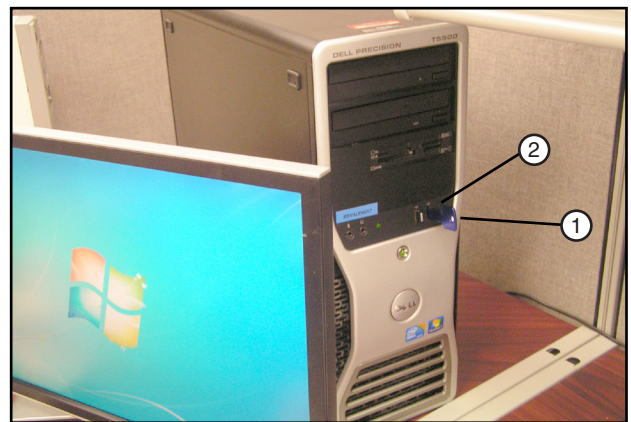
Figure 31-3 1. Flash Drive 2. USB Port
