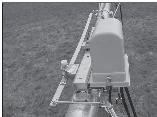
Figure 27-2 Modified Alignment - Adjustable Sensitivity
