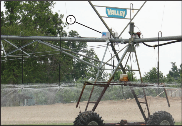
Figure 29-2 1. GPS Position Tower Box
