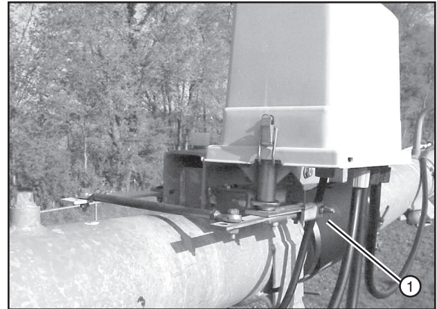
Figure 85-1 1. Tower box side of drive unit
