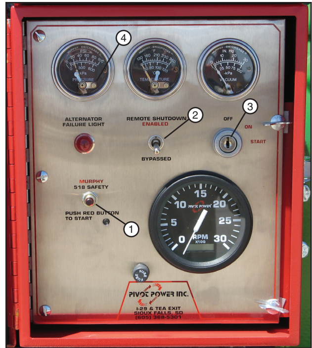
Figure 69-1 1. Safety Button 3. Engine Start Switch 2. Toggle Switch 4. Water Pressure Gauge Reset
