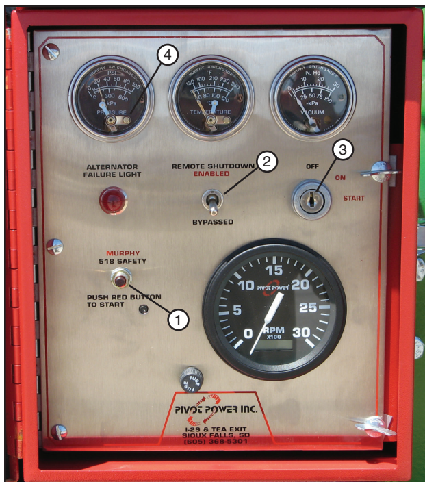
Figure 70-2 1. Safety Button 2. Toggle Switch 3. Engine Start Switch 4. Water Pressure Gauge Reset
