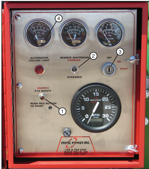
Figure 62-1 1. Safety Button 3. Engine Start Switch 2. Toggle Switch 4. Water Pressure Gauge Reset
