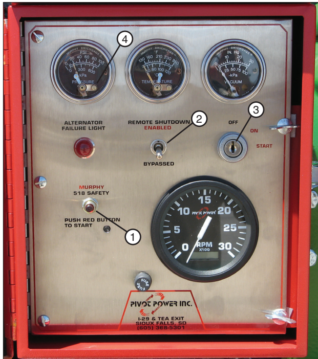
Figure 46-1 1. Safety Button 3. Engine Start Switch 2. Toggle Switch 4. Water Pressure Gauge Reset
