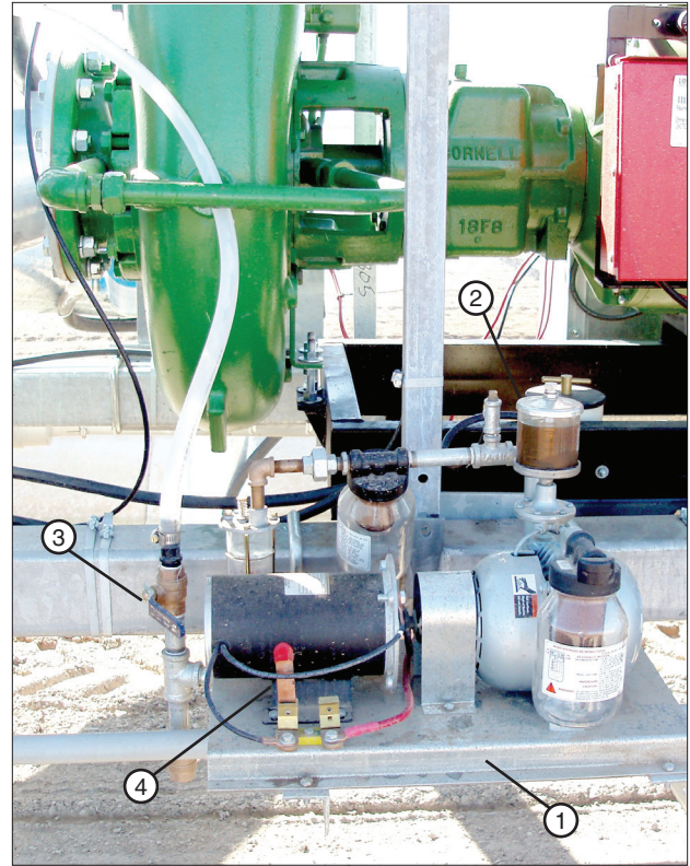
Figure 65-1 1. Electric Primer 2. Automatic Bearing Oiler 3. Ball Valve 4. Single Throw Switch
