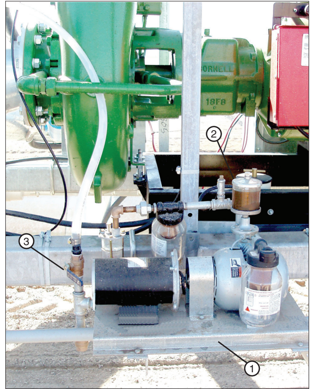
Figure 69-1 1. Electric Primer 2. Automatic Bearing Oiler 3. Ball Valve
