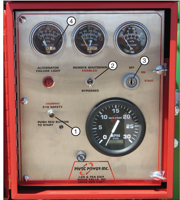
Figure 47-1 1. Safety Button 2. Toggle Switch 3. Engine Start Switch 4. Water Pressure Gauge Reset
