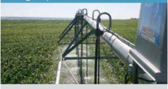
**Details:** The new longer span options help reduce the overall per acre installed cost by reducing the number of drive units needed. These 8000 series, 225-foot spans can also help to reduce the number of wheel tracks in the field for growers with track-prone land conditions. To learn more, talk with your local Valley dealer to find the best combination for your operation.
